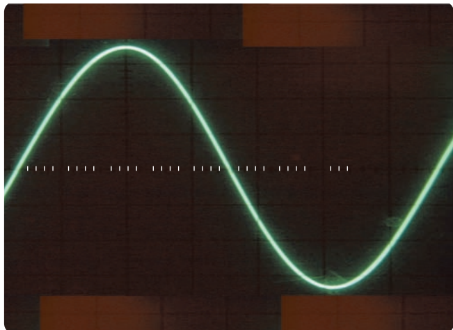
● Fig. 3: With the timebase set to 10 microseconds/div. And the Y attenuator to 1V/div., this sinewave would have a frequency of 10kHz and a peak amplitude of 3V.
