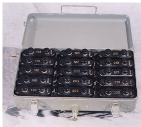
● Fig. 6: The 10RT's crystal selection housed in a sturdy case mounted on top of the receiver (see text).
