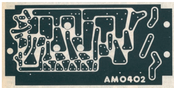
Fig. 5: Copper track side of the p.c.b. The actual size is 105 x 51mm (see text).
