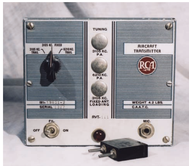
● Fig. 1: The AVT-111 Aircraft Transmitter. Ben says "It has nice simple clean lines" (see text).
