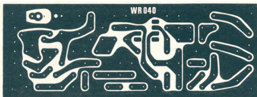
● Fig. 4: Full size printed circuit board design and associated component placement diagram.
