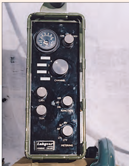
● Fig 4: The Pye Labgear LSP-30 h.f. radio, simple controls with clean lines (see text).
