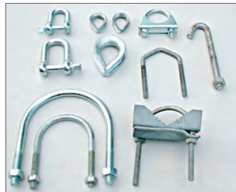
● Fig. 3: Various bits of metalwork to be found in good mast and antenna installation. Top-left are the D-shackles, with three 'eye-thimble' to their right. All of the items shown are available from marine chandlers or motor-parts suppliers.
