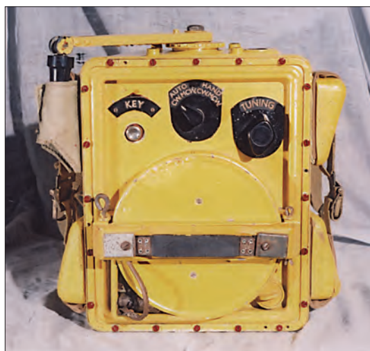
● Fig 2: The T1333 Emergency transmitter, crank handle stowed for transport. The drum carrying wire antenna is behind the central circular door.
