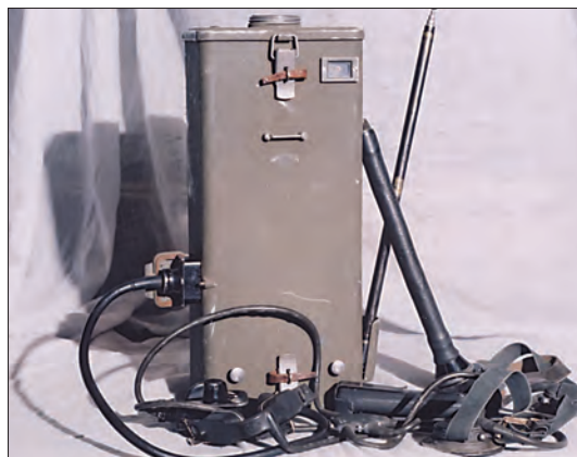
● Fig 3: The SE-103 Swiss walkie-talkie. The thick and thin antenna sections on the right screw together, and are mounted on top of the case when in use.
