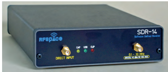
■ Fig. 1: The SDR-14 has no controls, not even a power switch, so it can be mounted out of sight. All the operational controls are in the software (see text).
