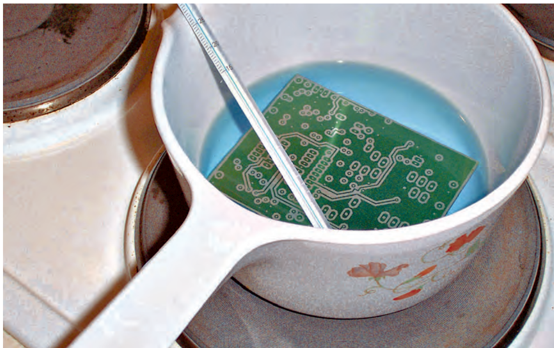
● Fig. 3 (right): A p.c.b. being etched in a non-metallic pan, most etchants have disastrous effects on normal household aluminium pans. This could lead to you becoming unpopular in the kitchen!
