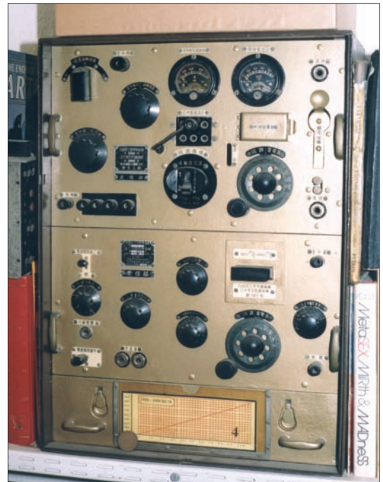
● Fig. 1: The 94 Mk III transmitter receiver, transmitter at the top, receiver in the middle with the receiver battery tray at the bottom. A fold down Morse key is on the right of the transmitter panel.
