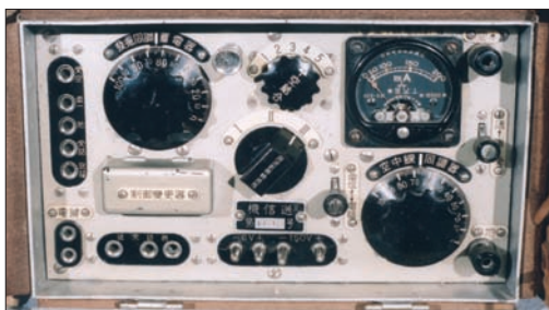
● Fig. 3: Close up of the Type 32 transmitter showing the meter and various tuning controls. The crystal is inserted under small cover lower left (see text).
