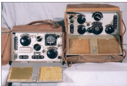
● Fig. 2: The 94 Mk V set, transmitter on the left, receiver on right (shown for size comparison).
