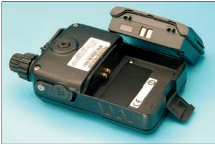
● Fig. 4: The transceiver can provide a full 5W output using the supplied battery pack (see text).
