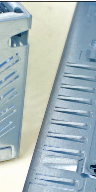
Fig. 1: Some PCs are much better screened than others. This one (an IBM ThinkCentre A30) has a two-part metal case. Notice the combs of springy teeth – over 80 of these all round the join ensure that little r.f. can leak out.
