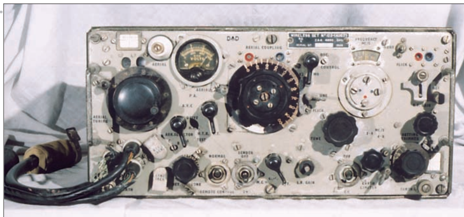
Fig 3: Wireless Set 122 (Aust), the main tuning is on the left, the large knobs centre and right are the antenna coupling and loading controls (see text).
