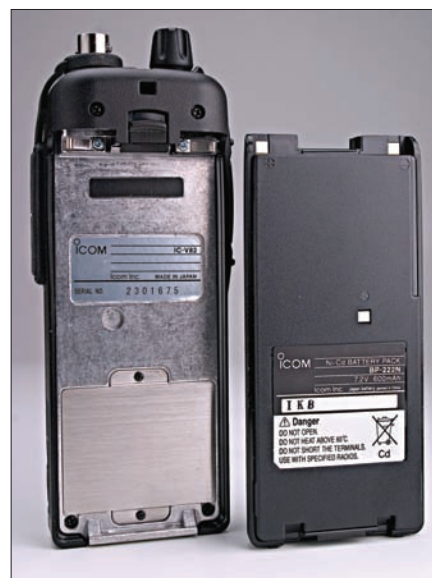
The detachable battery pack. The IC-V82 can only be powered by the battery pack, no external d.c. input socket is provided (see text).
