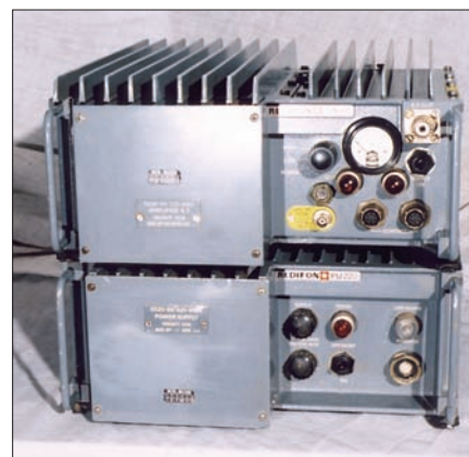
Fig 4: The Redifon GA481 100W amplifier and power unit. Note the substantial heat sink on both amplifier and supply cases.
