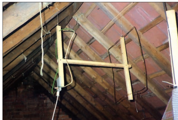
Fig. 3: The completed beam installed in the G3BDQ roof space.
