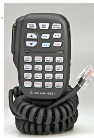
Fig. 3: The transceiver can be controlled from the microphone together with menu controlled memory addition and deletion. Even G3XFD found it user friendly! (see text).
