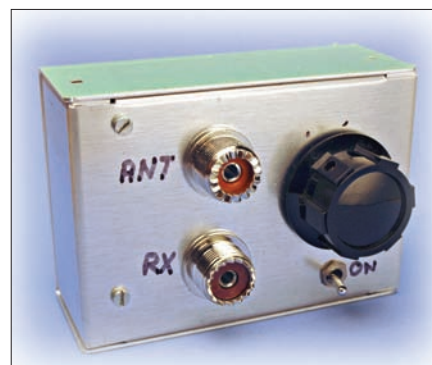
There's a noise bridge project to be built this month using zener diodes.
