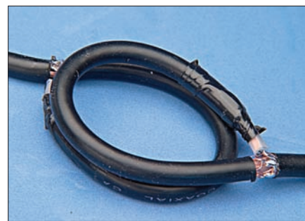
Fig.7b: A true 'braid breaker' filter before taping the loops together.
