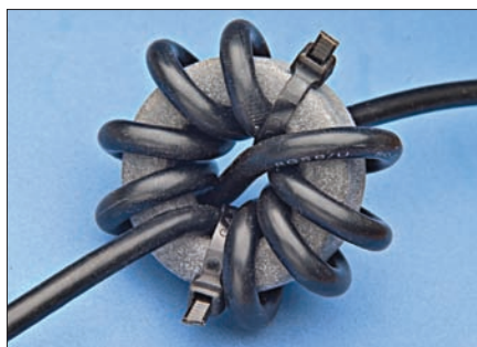
Fig. 7a: A practical 'braid breaker' design (in reality a choke filter). This is only one version! The coaxial cable could be wound as a solenoid and could be just as effective. There are many designs and G4LU recommends a good read of the many Amateur Radio manuals to find the design that suits your needs!
