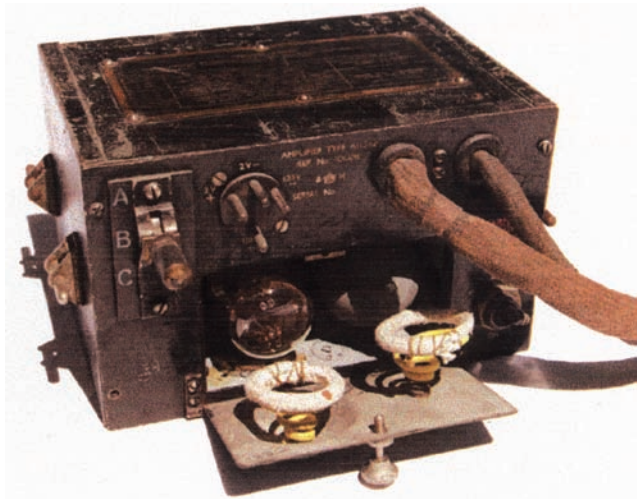
Fig. 4: Early bombers used the TR9F for r.t. (voice) communications, together with the A1134 or 1134A intercom (see text).
