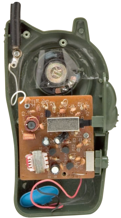
Inside the original radio. The Morse 'key' is low right on the p.c.b.
