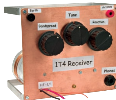
A simple regenerative receiver project.
