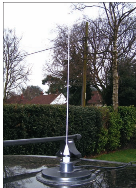
Fig. 2: Richard used a temporary magnetic mount to evaluate the transceiver and the whole assembly was installed in less than half an hour, although it was "not the recommended way to do it" says Richard! (see text).
