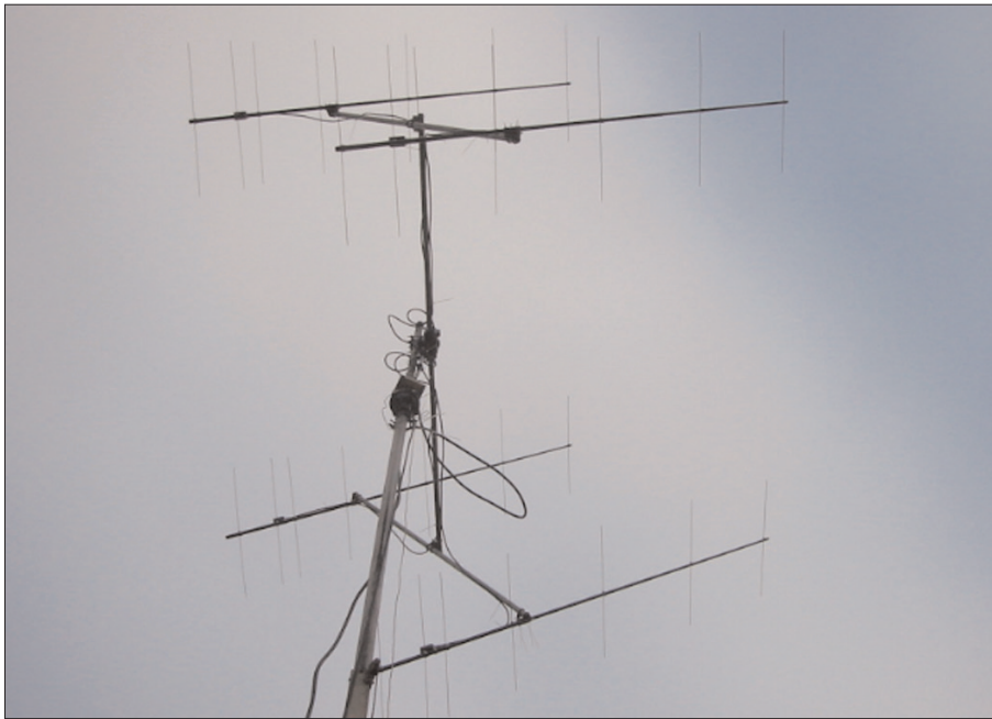
Fig. 1: The four by 7-element 144MHz array at the QTH of David Johnson G4DHF
