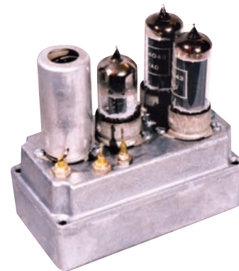
Fig. 4: The modulator sub chassis built on small Eddystone diecast box.
