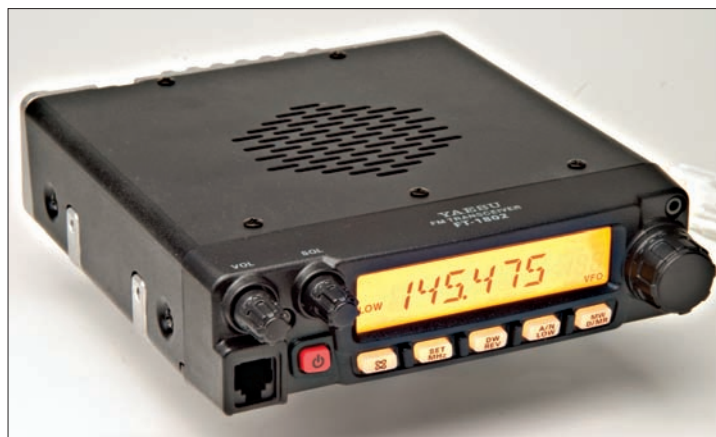
Fig. 3: General view of the FT-1802 f.m. transceiver, showing the large, clear display.
