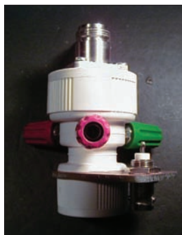
Fig. 11: Antenna mount and radial anchor.
