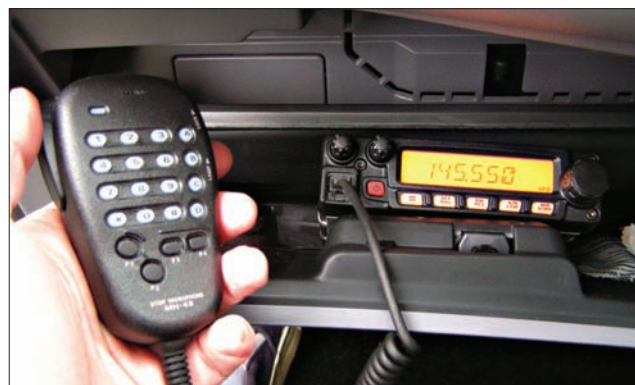
Fig. 1: As the FT-1802 does not have a demountable front panel/control head, temporary mounting site was found by using the glove box in GORSN's car. This photograph demonstrates how cramped the location was, but despite relying on convection cooling only, the FT-1802E showed no signs of distress. This view also features the microphone unit, the MH-48, which rather impressed GORSN in operation (see text).
