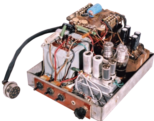
Fig. 5: The finished power supply modulator with matching rack connector.
