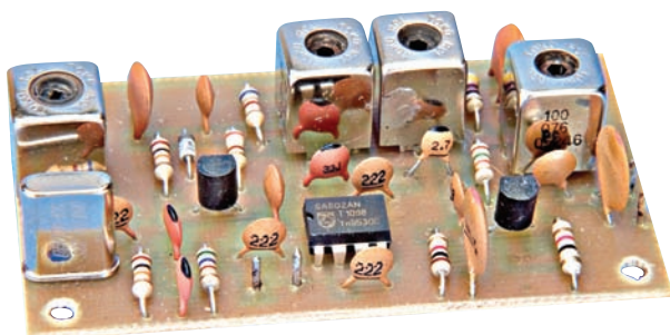
This month's project provides another step on the way to G4CFY's 70MHz s.s.b. transmitter.
