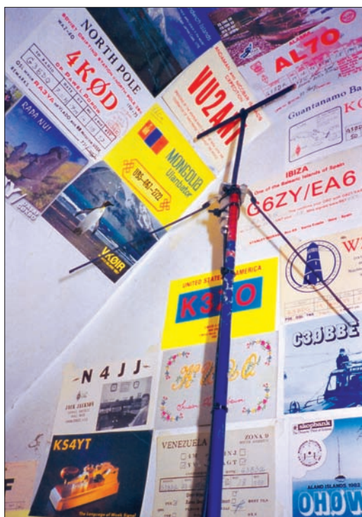
The T-Lambda fixed atop a two and an half metre pole. Its small size is obvious from the QSL cards in its vicinity.
