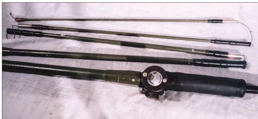
Fig. 2: The LSP-30 whip, tuning section with the insertable 4-section whip shown above (see text).
