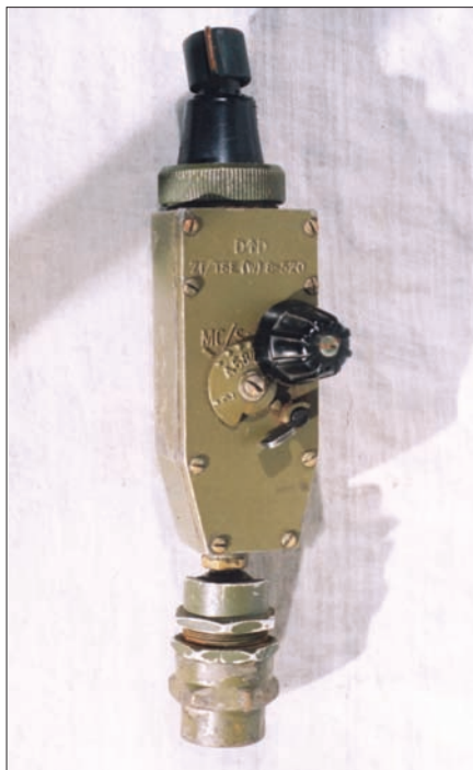
Fig. 6: The neat A510 whip tuner, marked 2-10MHz with a locking lever (see text).
