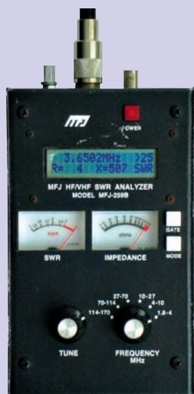
An antenna analyser. This one is the MFJ-259B; others include the MFJ-259Z, MFJ-269 and the Palstar ZM-30 antenna impedance bridge.
