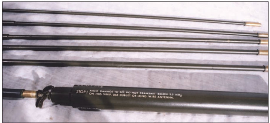
Fig. 10: The PRC-74 whip warning notice.
