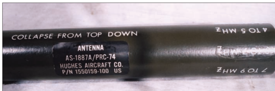
Fig. 8: The PRC-74 whip, with AS-1887A loading coil.
