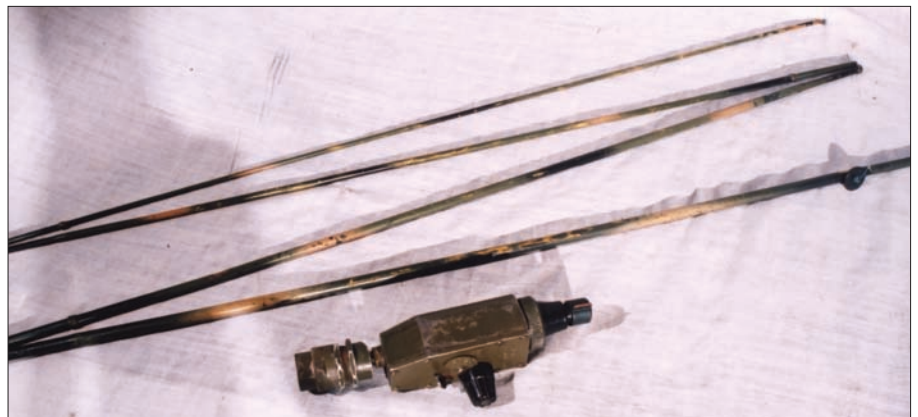
Fig. 5: The Australian A510 tuner and whip sections (see text).
