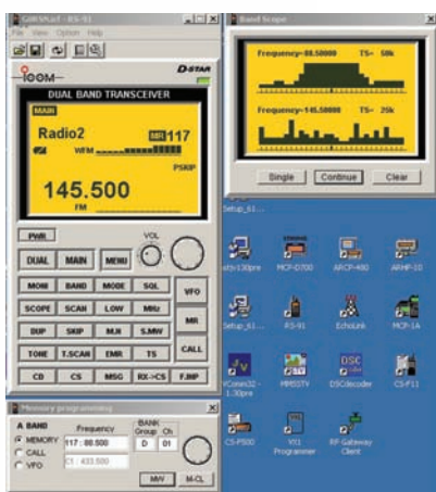
Fig. 3a: Richard GORSN installed the IC-E91 software on a Toshiba Satellite Laptop with an 800MHz processor and 512Mb of memory. The software installed without incident, and then he plugged the E91 in and immediately communicated with it.
