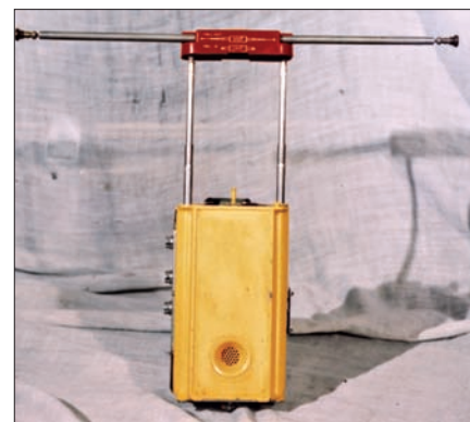
Fig. 3: The RT-159A with the antenna extended for u.h.f. operations. When operating on v.h.f. the two whips are fully extended (see text).
