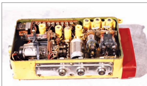
Fig. 2: Inside the RT-159A Survival set. The receiver on the left and the transmitter is on the right (see text).
