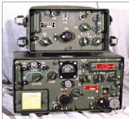
Fig. 1: The Chinese 102E station with transmitter (bottom) and receiver (top). There is a strong resemblance to the American GRC-9 radio styling and construction (see text).
