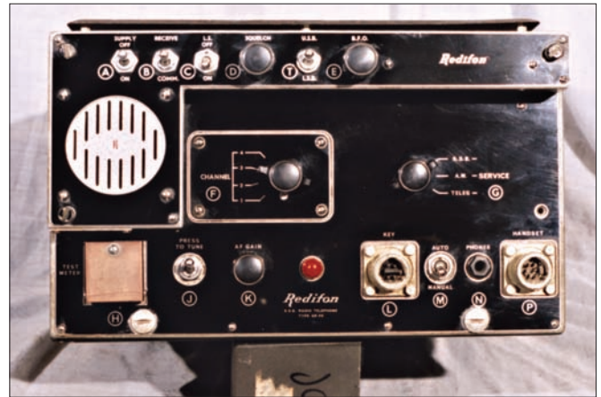
Fig. 5: The Redifon GR-410 marine transceiver, showing its very clean styling and simple controls (see text).
