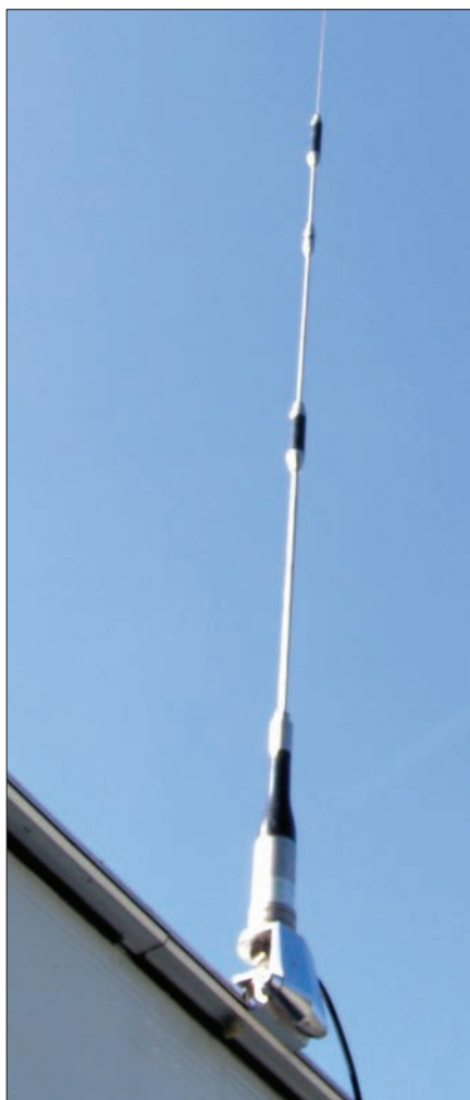
Fig. 5: During the on-air tests, Richard attached a high gain, dual-band mobile whip to the metal guttering of the holiday caravan (see text).
