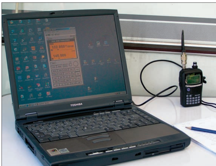
Fig. 3a: Richard GORSN installed the IC-E91 software on a Toshiba Satellite Laptop with an 800MHz processor and 512Mb of memory. The software installed without incident, and then he plugged the E91 in and immediately communicated with it.
