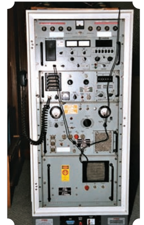
Fig. 10: A superb synthesised Harris Receiver and transmitter h.f. base station. Made in the USA, the Harris RF-550 receiver and its associated transmitter. This version was (possibly) made in the early 1980s and tunes from 10kHz to 29.999MHz in 100Hz increments. The receiver includes c.w., a.m., l.s.b., and u.s.b. It can also receive and demodulate independent sideband (i.s.b.) - differing intelligence on each sideband. It was designed for special, highly congested tactical condition working 'in the field'.
