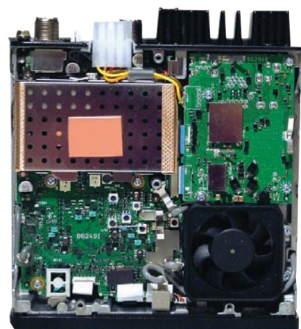
Fig. 9: Top chassis view, with the cooling fan on the right.
