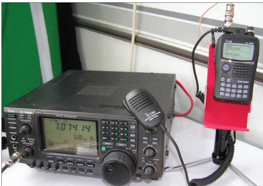
Fig. 6: The operating position in GORSN's caravan. The first two contacts were made using the IC-E91 while it was connected to the mobile whip on the caravan's guttering.
