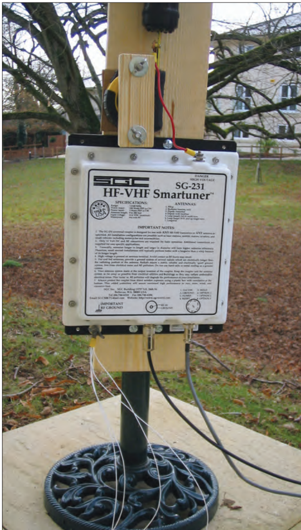
Fig. 6: The arrangement described in Fig. 5 also provides a suitable support for fixing the antenna to the base of a patio umbrella stand for use on the patio.
