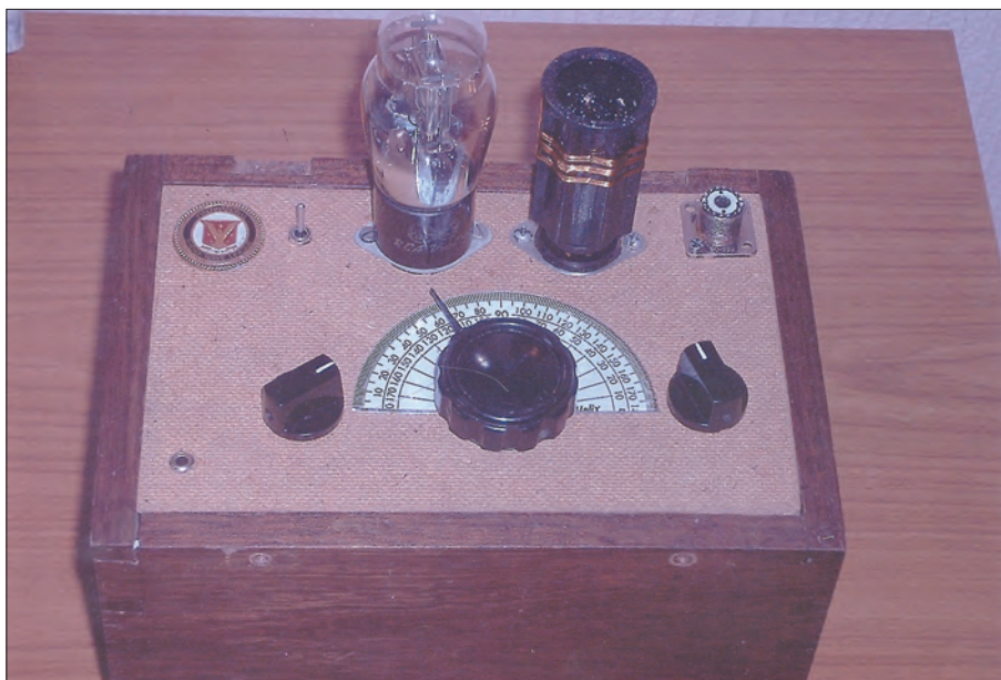
Fig. 2: Reader Ron Pearce has built a Hiker's One. The set covers 1.8 to 28MHz using three plug-in home brewed coils and uses a genuine type 49 valve (see text).
