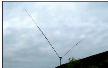
Fig. 4: The Comet H422 rotary dipole - assembled in the V configuration - ready for use (see text).
