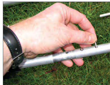
Fig. 2: The traps on the antenna need to be carefully located on the assembly (see text).
