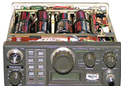
The Yaesu FT-290 uses eight 1.2V 2A hour NiCad batteries, a total of 9.6V.
