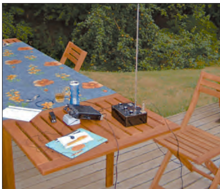
Roy Walker F/G0TAK's portable station using a Yaesu FT-817 and MFJ-1621 portable antenna
