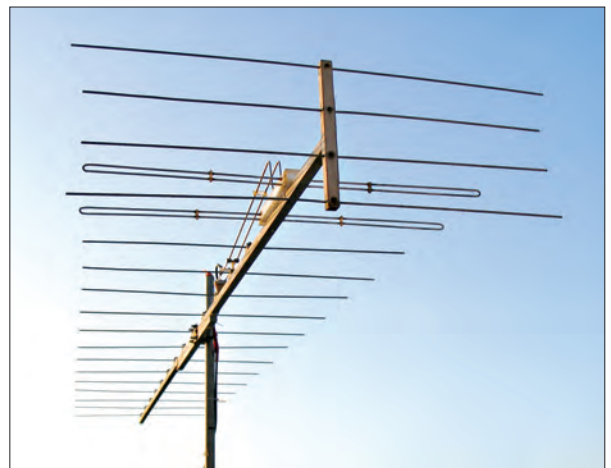
Fig. 1: Photograph of the G2BCX antenna, built by John G8WOW. This view shows the two driven elements.
