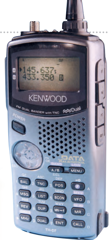
Fig. 1: The Kenwood TH-D7E has many features that Peter G4AJG considers to be very useful for use when working via Amateur Radio satellites.
