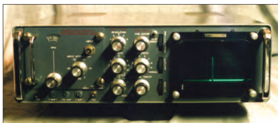
Fig 5: The Eddystone EP-961B display unit, showing a 500kHz calibration pip.
