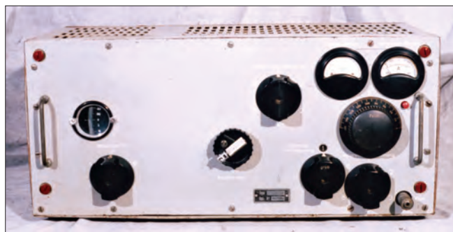
Fig. 3: The German Naval transmitter, tuning window on the left, with the power amplifier and antenna controls on the right.
