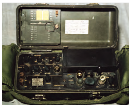
Fig. 2: The PRC-64A transmitter receiver. The battery is housed under the cover top right of the set.
