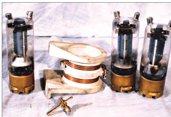
Fig. 4: The valves and oscillator coil out of the LO40K39, the stuck shaft (see text) was removed and repaired.
