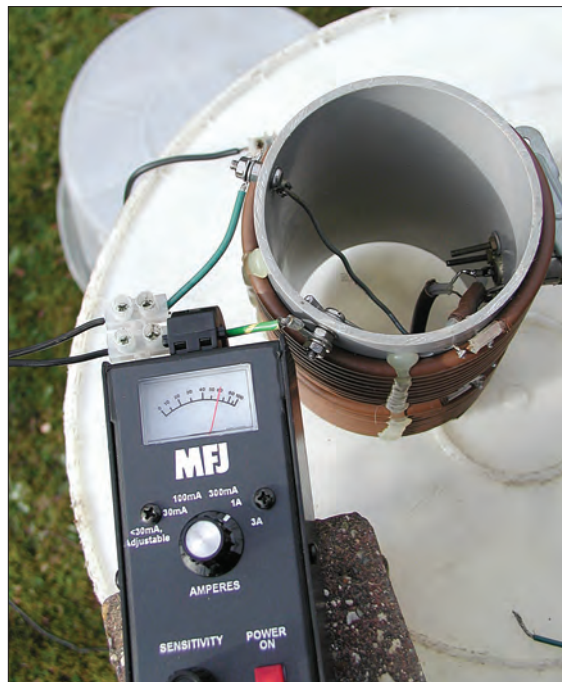
Current measurements on the twin feeder conductors (telephone line) to OCFD. A PA0SE coaxial balun is used to match the twin feeder to the coaxial cable feeder.
