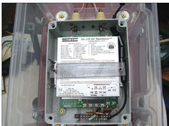
Fig. 3: The SGC SG-239 a.a.t.u. mounted in its box, ready to be sealed into the external casing.
