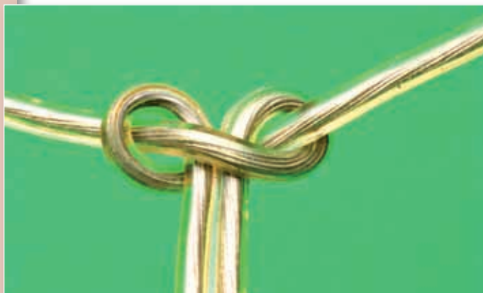
Fig. 1: The special 'Electrician's' knot used to fix the dipole feed-point when using figure-of-eight cross section flexible cable.
