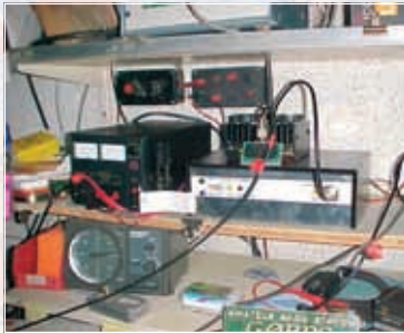
Situated in the home shack of GOBPS. The final transmitter in the alloy box, the p.a. is shown above with the temperature sensor.
