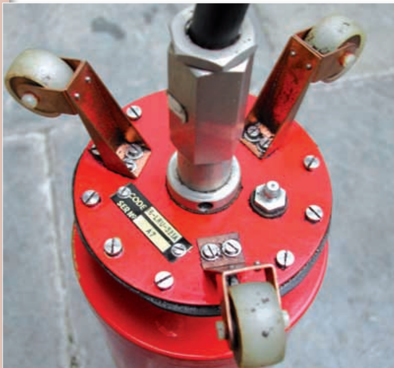
Fig. 1: The canisters, hanging on cable, were kept 'steady' within the tubes with the help of spring loaded wheels.
