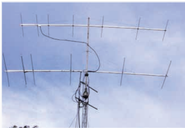
The 70MHz 7-element Yagi antenna that's featured this time, above a 50MHz 6-element Yagi.
