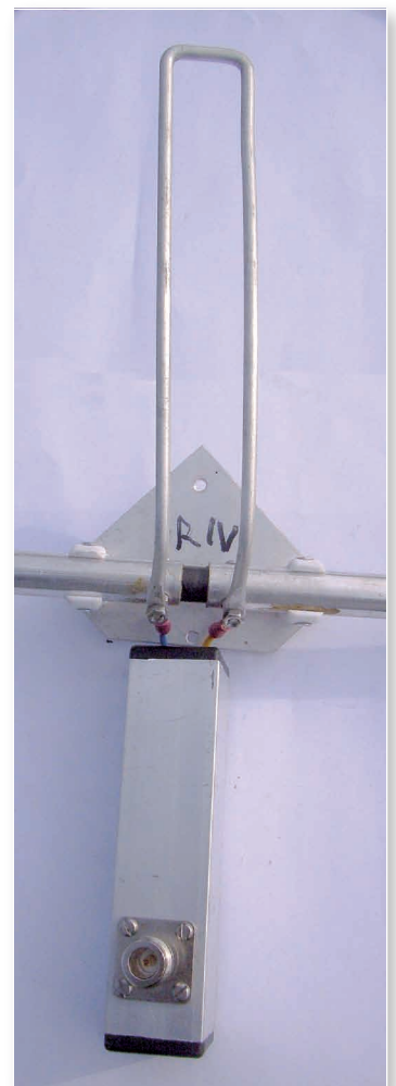
Fig. 5: The Hairpin Match & Balun Assembly.
