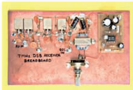
Fig. 2: As part of the development process, Tony G4CFY used an amplifier built for the earlier DiBD audio amplifier article. He added it to the copper clad breadboard as shown here.
