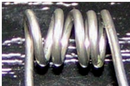
Fig.4: A replacement coil for an FT-225RD, wound on a 2.5mm mandrel.
