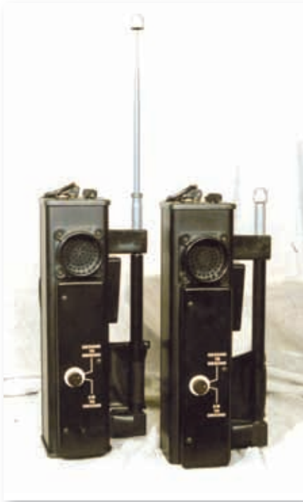
Fig. 3: The Vietnam war era HT-2 walkie talkies with extra long whip antennas.
