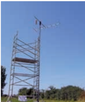
Fig. 2: A 20m high scaffolding tower ensured the antenna system was well clear of obstructions, providing a horizon-to-horizon pathway for the QSO.
