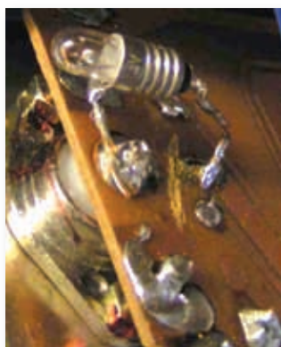
Fig.5: Adding a 6V/100mA bulb to the output socket of your signal generator, should protect it if you inadvertently transmit into it.
