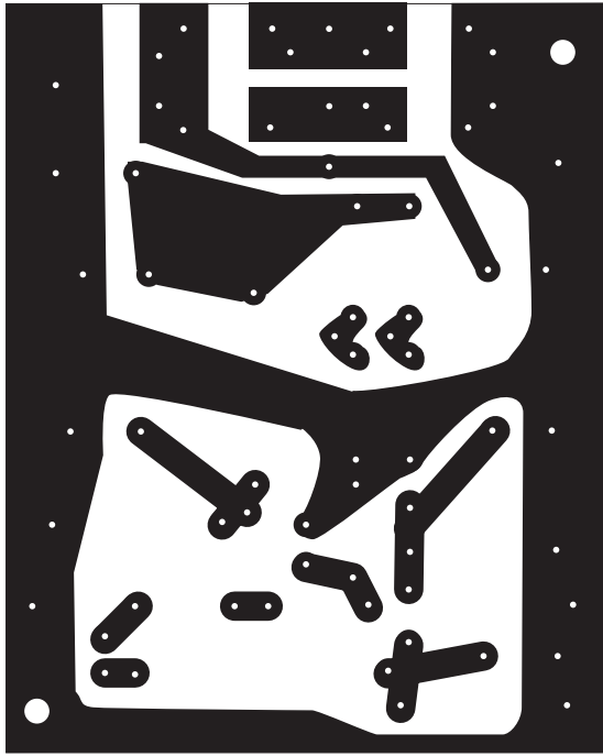
Fig. 2: A suitable printed circuit board, showing the track and component overlay.
