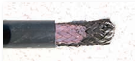
Fig. 2: The result of water entering the outer insulation of a section of coaxial cable and corroding the screen. Severe mismatch and its attendant losses can occur when this happens.
