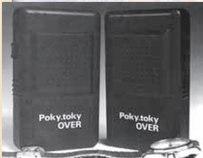
The Poky-toky OVER was actually supplied as a matched pair of transceivers.
