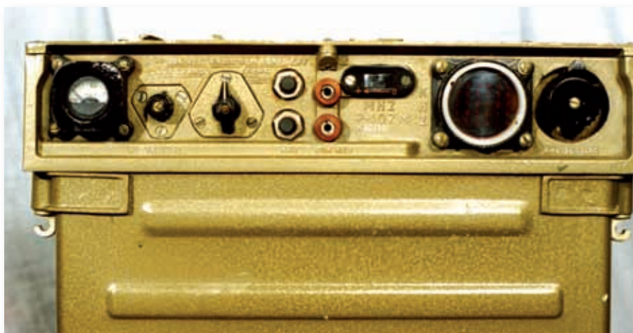
Fig. 2: The P-107M controls, two tuning dials, MHz centre right, kHz in the round window.
