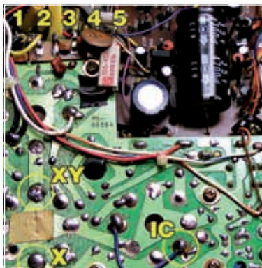
Fig.3: The new resistor is added to the right-hand terminal, marked 5.
