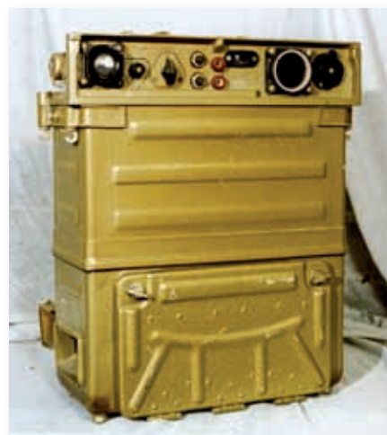
Fig. 1: The Russian P-107M man-pack set, batteries fit in the base of the unit.
