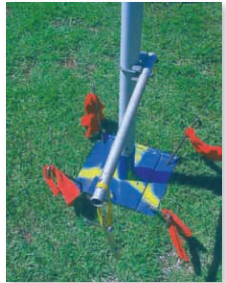
Fig. 2: The VJK5AIM mast base with warning flags for use on caravan sites. The 'Armstrong' mast rotating system is shown mounted at waist height, complete with safety marker to ensure caravan site users don't walk into it.
