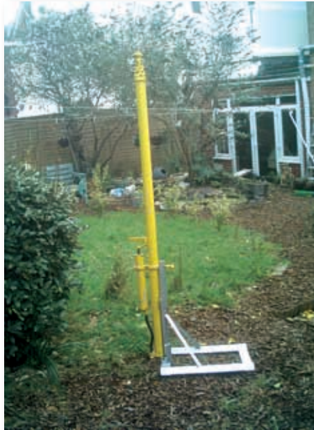
Fig. 1 (far left): The modified Tenna-Tourer mast base.
