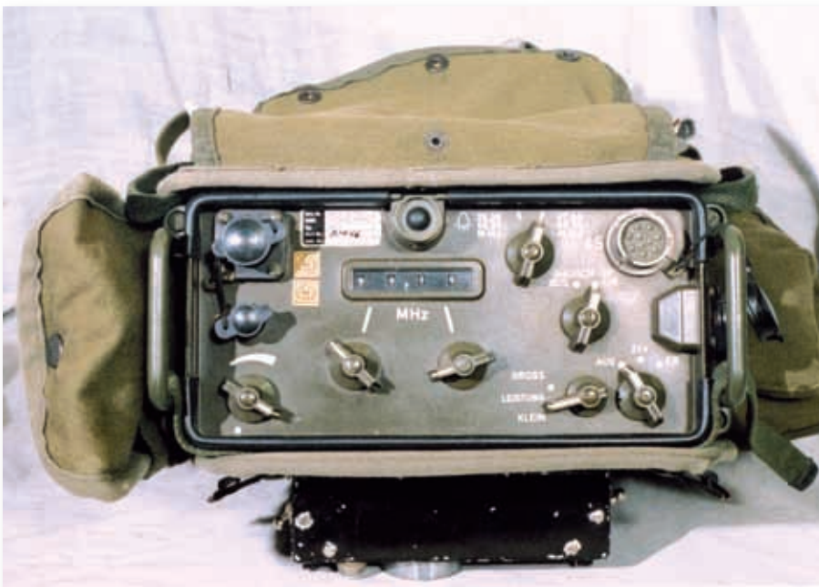
Fig. 4: The SEM 35 v.h.f. man-pack set, with the mechanical digital frequency display in the centre.
