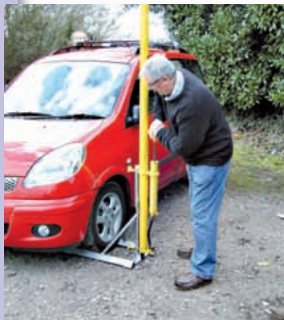
Fig. 1: The GB75PW Special Event Station took advantage of G3XFD's car as a base mount for the antenna. Because the crew forgot to lock the sections up as they were erected they spent much time re-pumping air into the mast! (Lesson learned – lock the sections as the mast is erected!).
