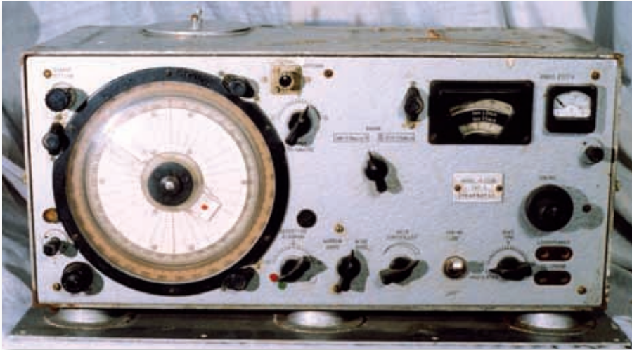
Fig. 3: The Russian DF receiver, the direction bearings are indicated by the large left hand dial.
