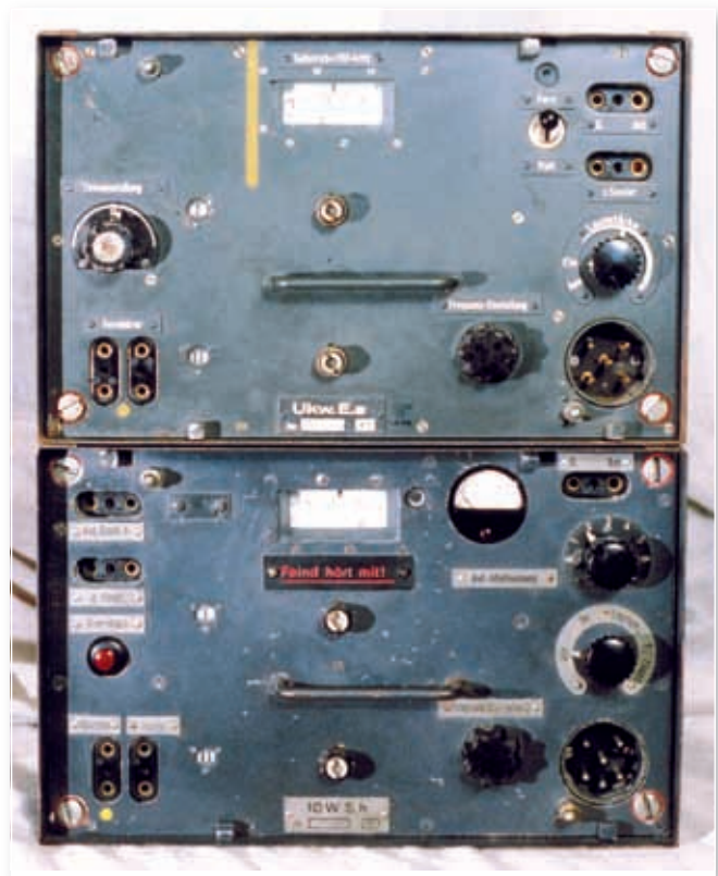
Fig. 1: The Ukw E.e receiver (top) with 10WS.h below, now operating on 28MHz.
