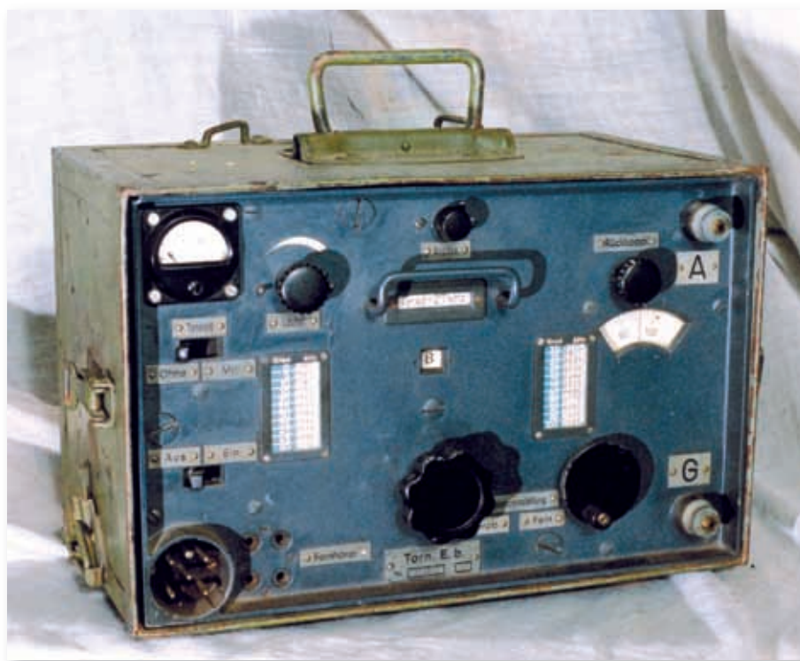
Fig. 2: The Torn E.b receiver, the charts in the two windows change as the band switch is rotated.
