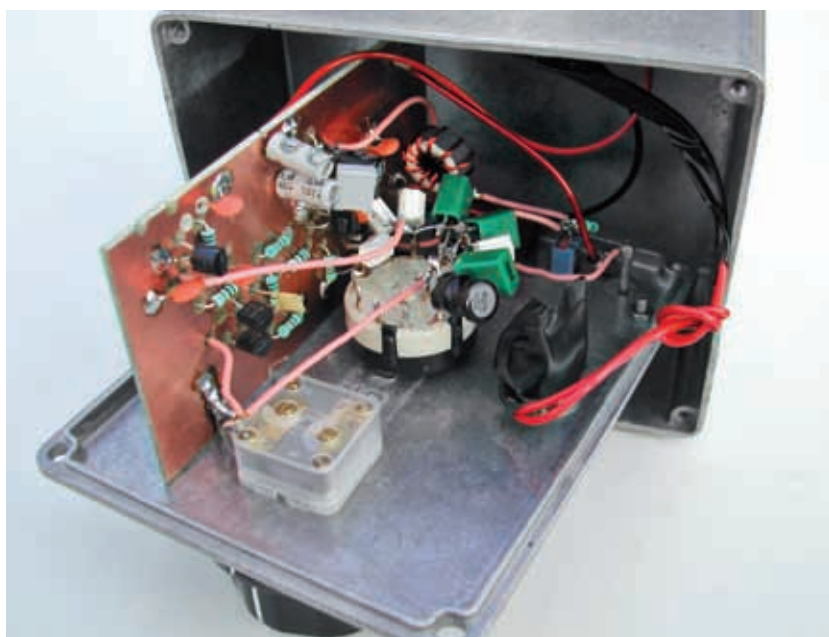
Photographic montage showing the signal generator project built 'open style' (top) and assembled into a dye cast aluminium box (below).
