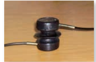
Fig. 4: Making a 'transformer' with two telephone pickup coils.
