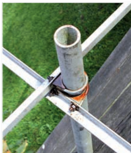
Fig. 7: A method of constructing a robust spider for a large quad using angle aluminium and car exhaust clamps.
