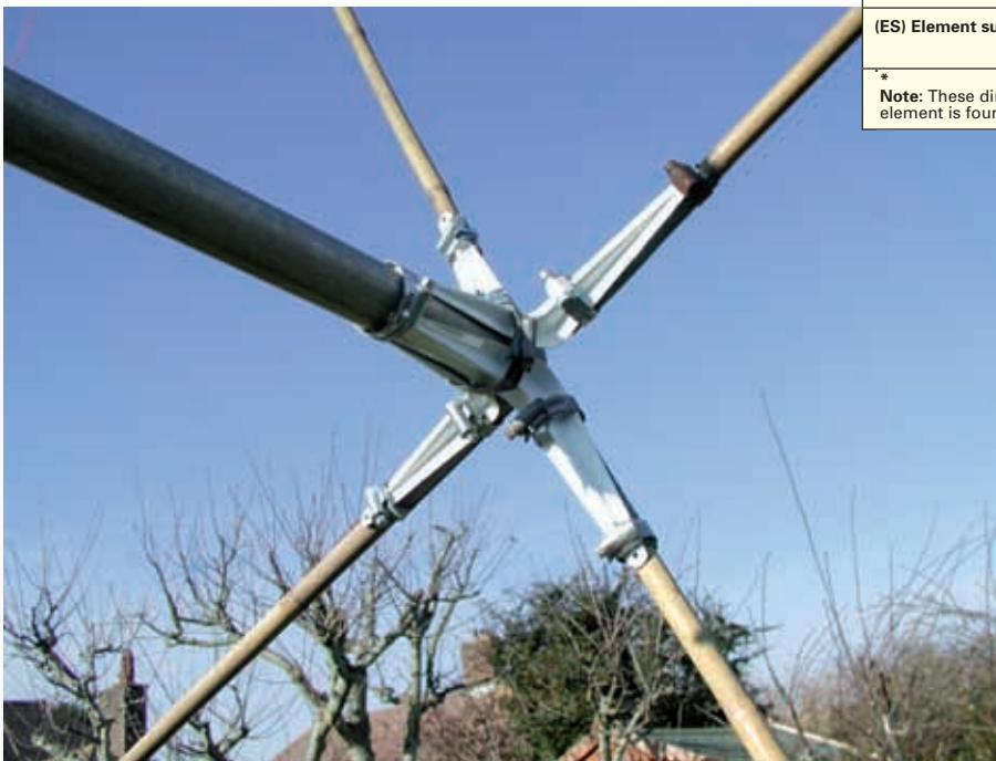
Fig. 5: Method of fixing the shelf brackets to the boom using Jubilee clips to construct a spider.
