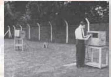
Showing the new instrument known as EVA (Electronic Velocity Analyser) for measuring speeds of guided missiles.
