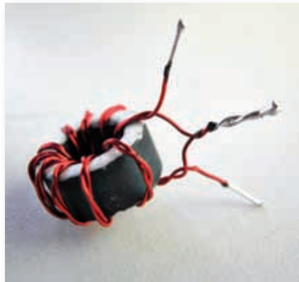
Fig. 2: Close up view of toroid inductor L9.
