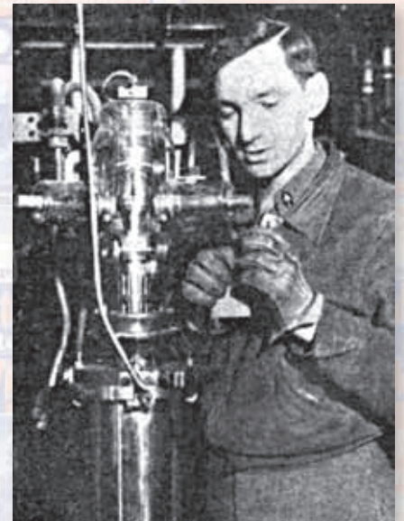
After going off the air when the Germans advanced into Luxembourg, this station was dismantled, but started operating again at the end of last December. The illustration shows a radio engineer making a final connection to one of the high-power valves.
