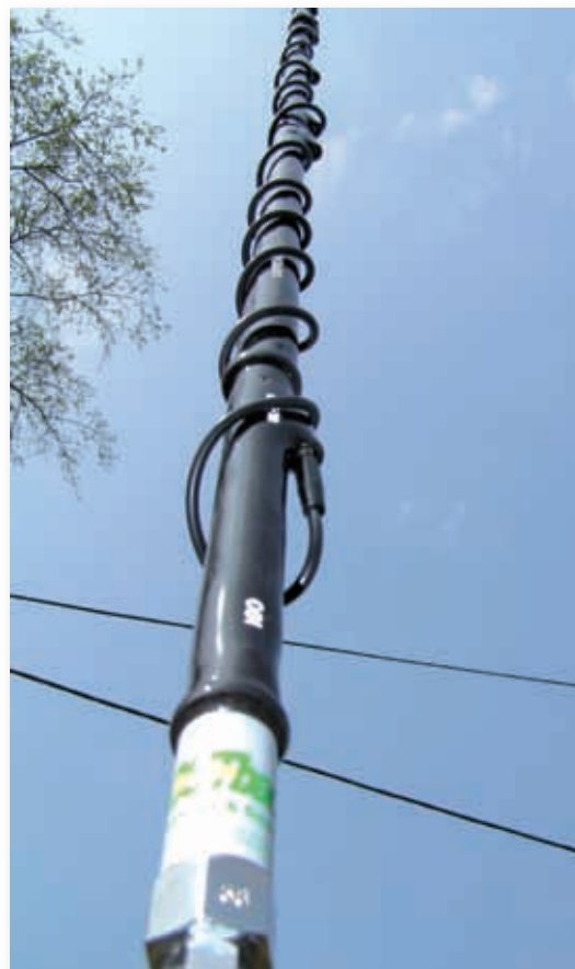
Fig. 2: The wander lead curls around the antenna and connects to the appropriate band match point.
