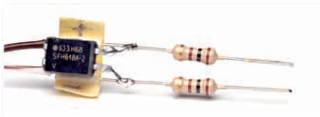
Fig. 8: A suitable CAT programming interface. The resistors do not interfere with the process but have leads suitable to fit into the rig's socket.
