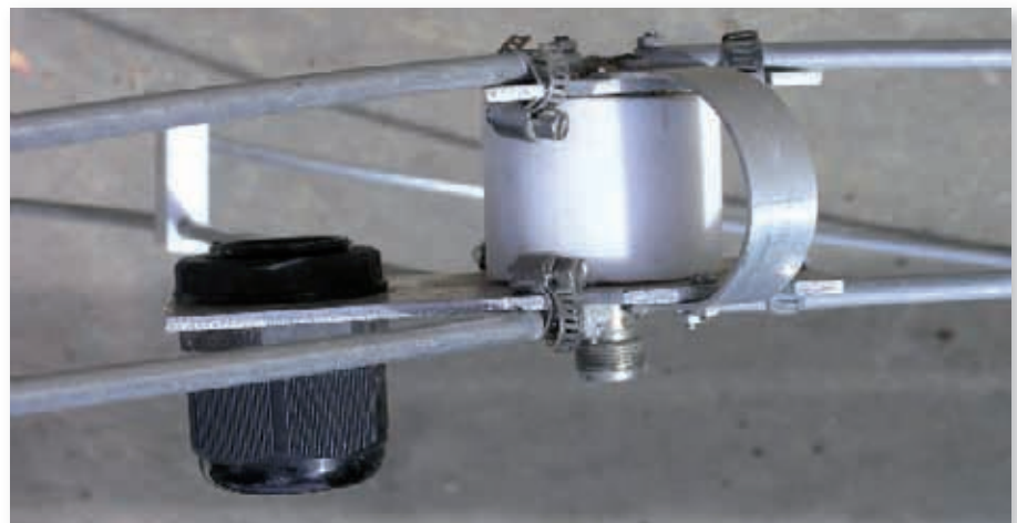
Fig. 5: The centre clamping plate and 'hairpin' match.
