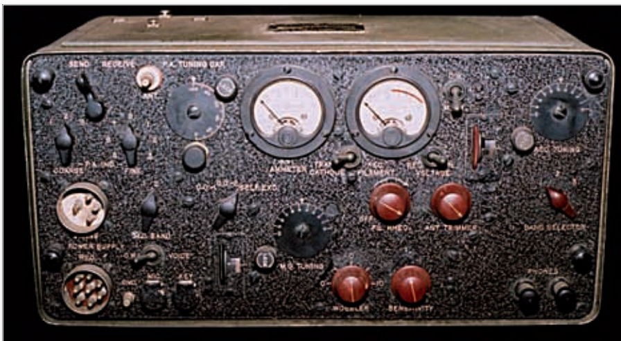
Fig. 3: The TBX-2 transmitter receiver, transmitter, tuning centre and receiver tuning, visible at the top right.
