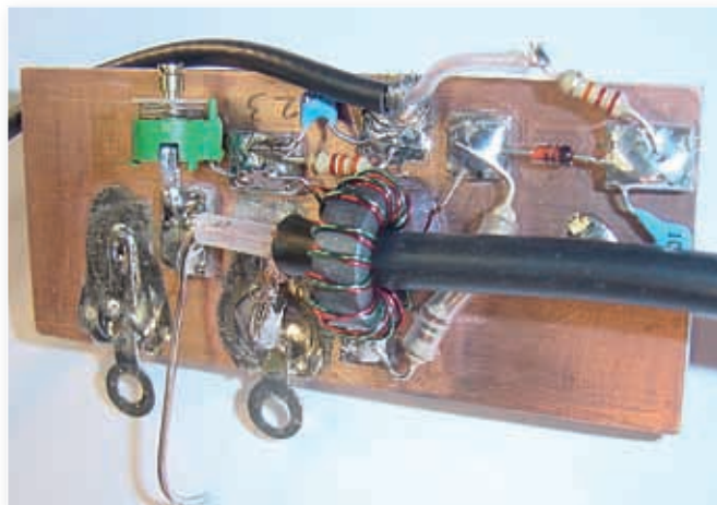
Fig. 5: Bridge board ready for installation. The protruding solder lugs will be bolted and grounded to the inside of the SO239 socket on the rear panel. The thin coaxial cable (to the left) leads to the front panel meter M1, the cable to the right goes to C1.
