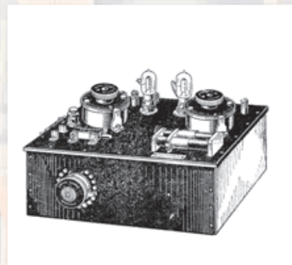
Fig. 3 – In this illustration we see one of the early valve receivers employing two Fleming diode valves. The circuit employed only a single valve, but two were fitted in the interest of reliability, and a switch enabled one or the other to be brought into circuit. Note the massive variable condensers, and compare them with modern components. The dielectric employed in these condensers consisted of plate of thick ebonite, but the components were very efficient.
