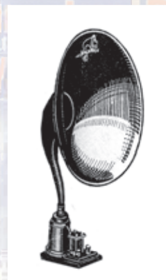
Fig. 9 – One of the earliest and at the same time one of the most popular loud speakers – the Magnavox. This employed an energised magnet requiring an applied voltage between 6 and 10 and the diaphragm was of the conical type. This was operated by a moving coil and was used on many occasions for public address demonstrations.
