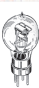
Fig. 5 – The well-known French ‘R’ valve. This was extremely popular amongst amateurs immediately after the war, but its performance would be extremely poor compared with modern valves. It formed an ideal detector and was used in its thousands.
