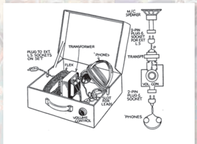
A good scheme to enable headphones or loudspeakers to be used at will. This arrangement is particularly valuable in the case of illness.
