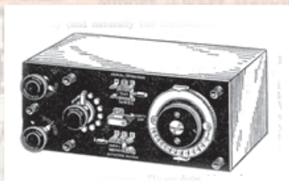
Fig. 2 – An early army-type tuner. This was designed for use during the early days of the Great War, and employed a flat tuning inductance arranged to tune after the manner of a variometer. Switches were provided to enable the detector and phone to be joined across either the "closed" or the "aerial" circuit.
