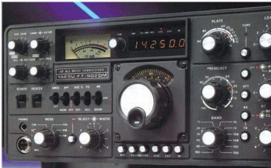
The FT-902 was an upgraded version of the FT-901 and featured an improved r.f. board and frequency counter.
