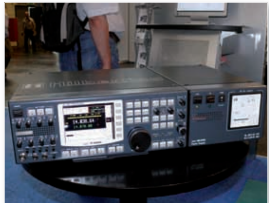
The innovative German designed and built Hilberling PT-8000A h.f./v.h.f. 100W p.e.p. transceiver created a lot of interest when it was first shown last year and the latest version has a host of new features. More details (in German) can be found at: www.hilberling.com or in badly translated English at: http://translate.google.com/translate?hl=en&sl=de&u=http://hilberling.com/hamrad/hamradio.htm&sa=X&oi=translate&resnum=2&ct=result&prev=/search%3Fq%3Dhilberling%26hl%3Den%26rlz%3Dcom.microsoft:en-us:IE-SearchBox%26rlz%3D117DKUK
