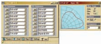
Fig. 21: The first skip distance depends on the low-angle radiation capabilities of the antenna.
