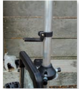
Fig. 11: The field strength meter sits on a small plastic bracket on the vertical element of the antenna.
