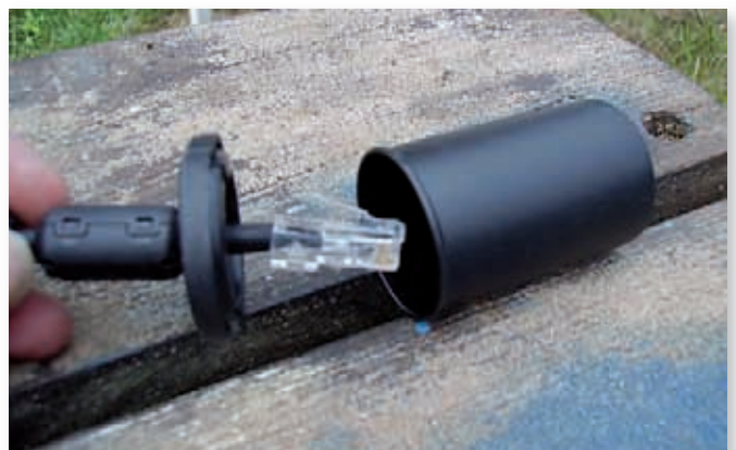
Fig. 14: The microphone plug about to be fitted into the storage container made from a 35mm film canister.
