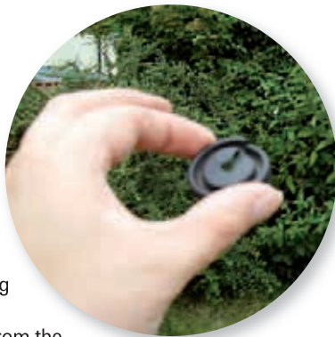
Fig. 15: a closer look at the hole and slot cut into the canister's lid.
