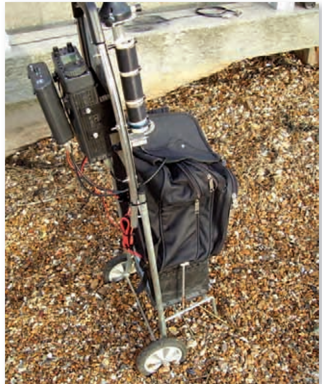
Fig. 2: the rig, automatic tuner and manual tuning components in action at the top of the trolley.
