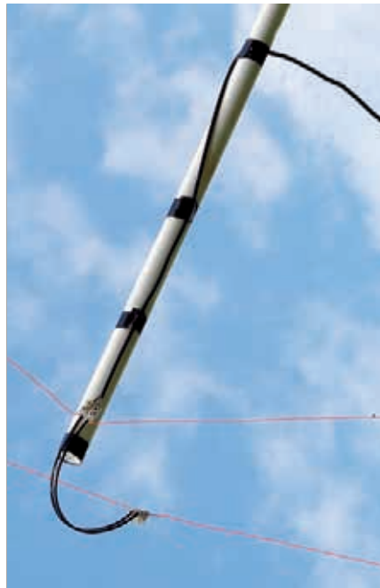
Fig. 2: The feeder support arrangement uses a plastic tube. This arrangement holds the feedpoint in place and holds the feeder clear of the mast when the antenna is used on the lower frequency bands. 'Choc-block' connectors are used as insulators and for fixing the ladder line to the elements.
