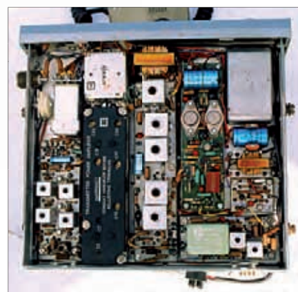
Fig. 4: Peering from above at the insides of the 'Wessie' shows the modular construction methods used.
