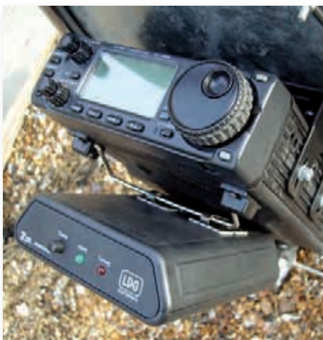
Fig. 17: The Z100 swung away from the body of the rig so, that you can see the clips mounted on the upper side of the tuner unit.
