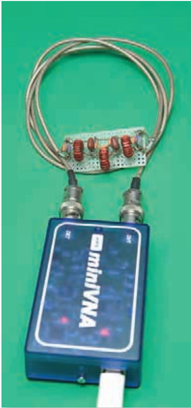
Fig. 8 (left): And here's how the set-up looked when measuring the filters.
