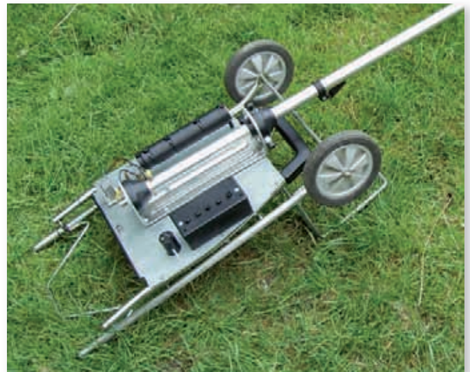
Fig. 3: The antenna base mounting plate is fitted to the fold-over handle.
