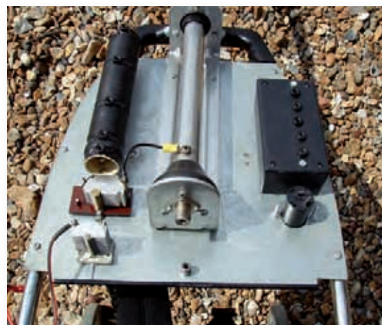
Fig. 7: A closer look at the antenna mounting plate with the two tuning capacitors and the base-loading coil on the left-hand side.
