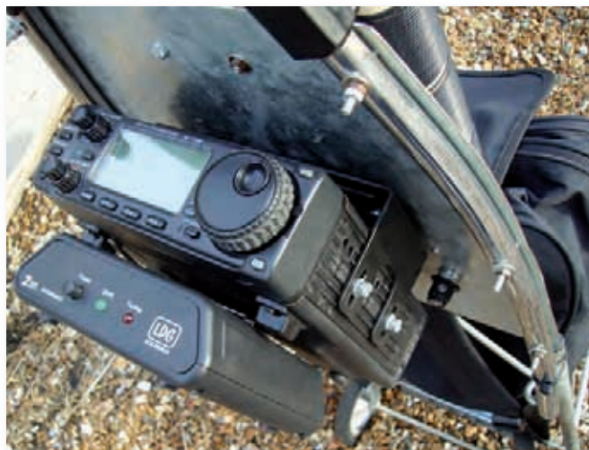
Fig. 16: The LDG Z100 automatic antenna tuning unit in the 'normal' operating position.
