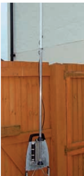
Fig. 7: A closer look at the antenna mounting plate with the two tuning capacitors and the base-loading coil on the left-hand side.
