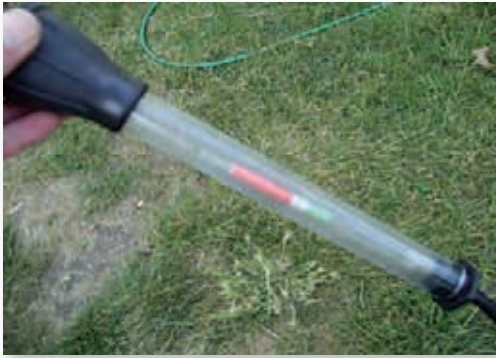
Fig. 9: The hydrometer's density scale gives a better indication of the effective states of individual cells in a battery.
