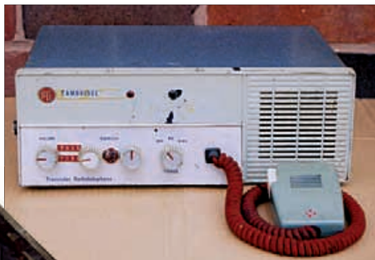
Fig. 2: A little younger than the Reporter of Fig. 1, the Cambridge , still had a valved transmitter but had a transistorised receiver.
