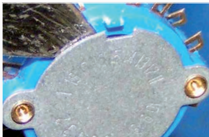
Fig. 2: By easing the plate away from the body, a small amount of switch cleaner can be squirted into the contacts.
