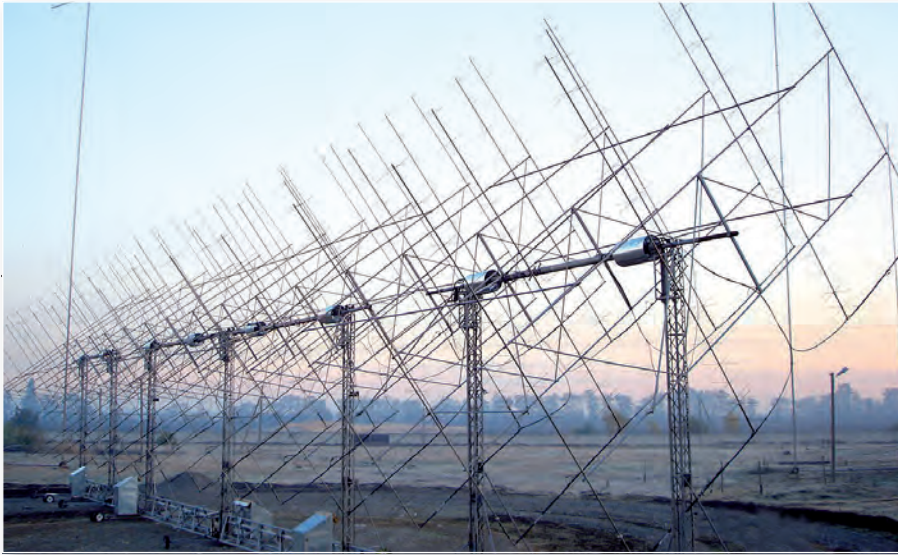
The impressive array of Sam Sam Dubovtsev RN6BN with 64 combined 15-element Yagi antennas for 144MHz e.m.e. working. This is, as you might expect, the world's largest array for e.m.e. work on 144MHz.
