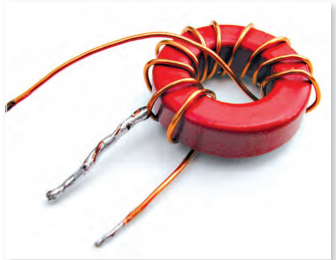
Fig. 4: A toroid wound for the 14MHz band.
