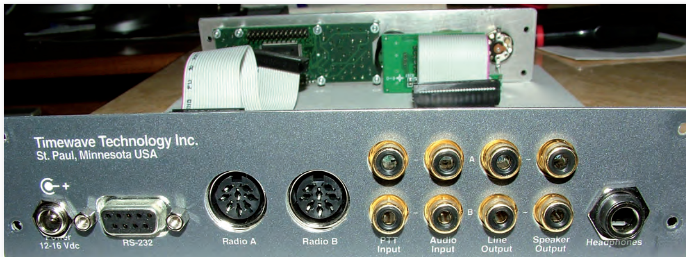
Fig. 2: A closer look at the input and output connections and the two radio connections.
