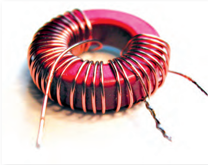
Fig. 3: A toroid wound for the 3.5MHz band.
