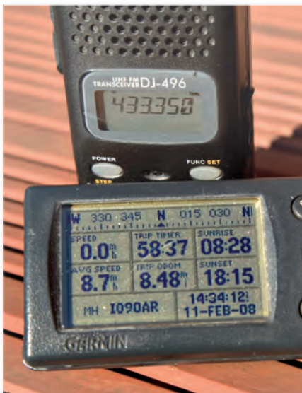
Fig. 4: Some GPS units, such as the Garmin GPSIII, make it easy to find your locator as shown in the lower left section of the display.
