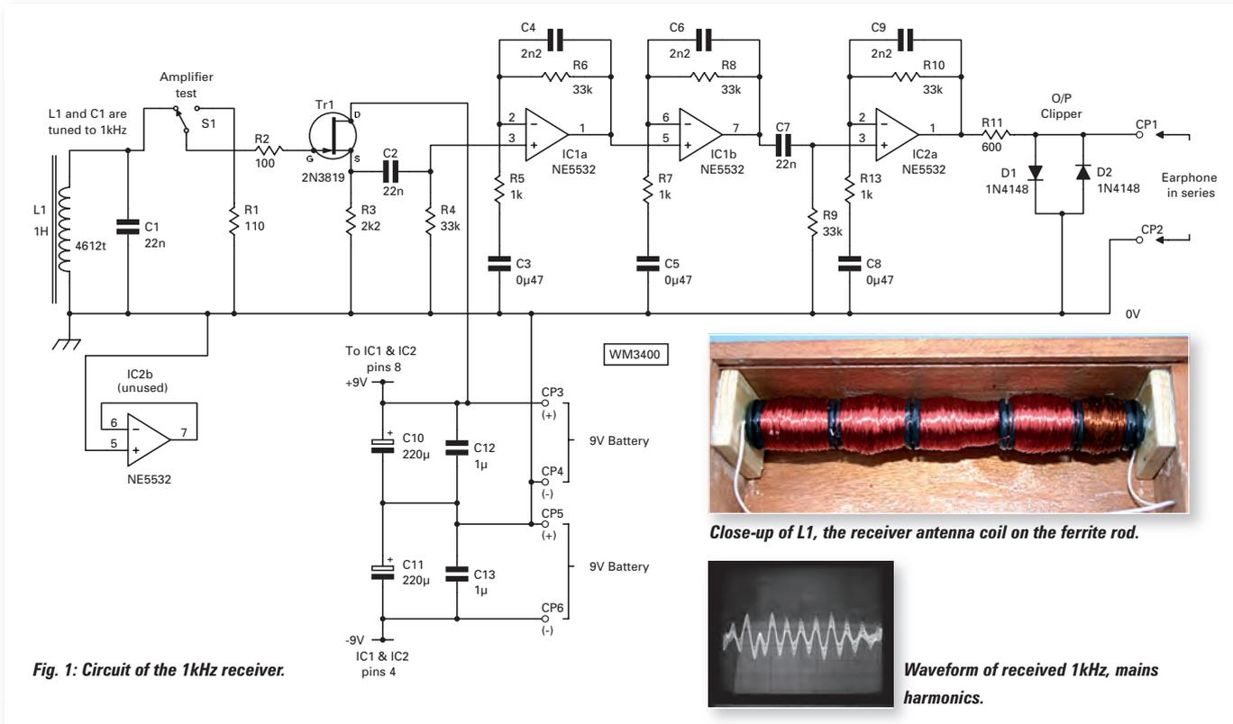
Fig. 1: Circuit of the 1kHz receiver.
