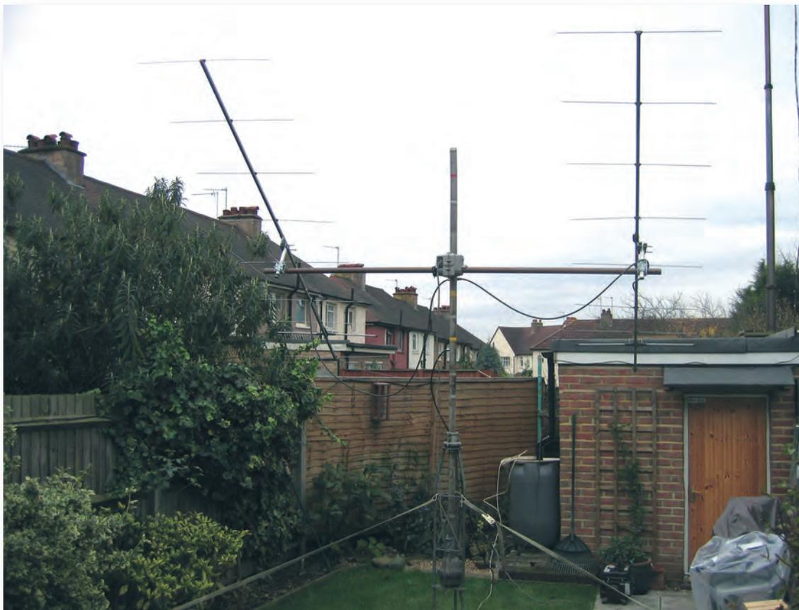
**Fig. 2: The 144MHz antenna array of Simon Smith 2E0VAG.**
