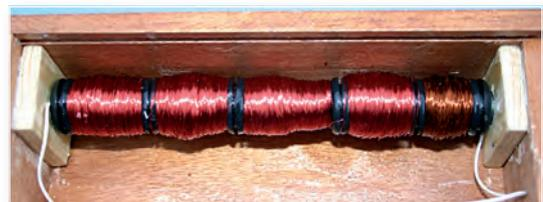
Close-up of L1, the receiver antenna coil on the ferrite rod.
