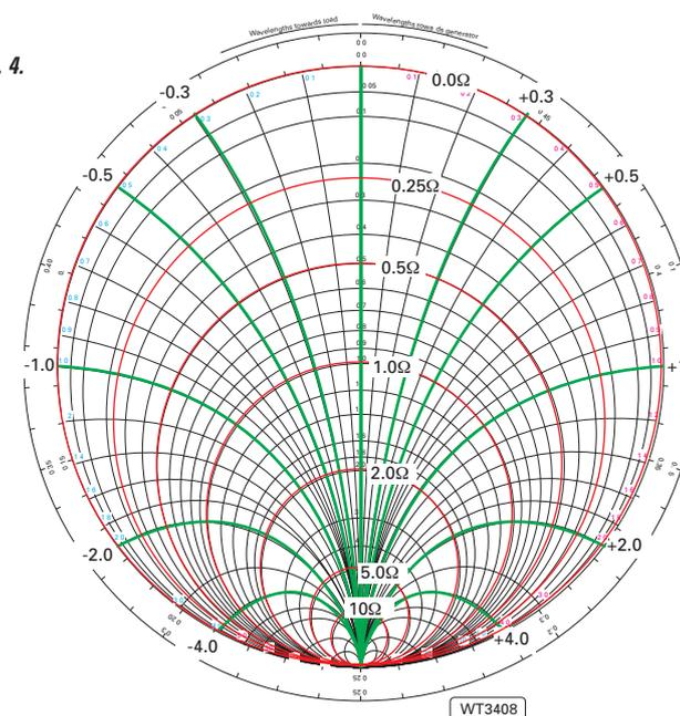
it's a measure of **distance**, not in metres or yards, **but in fractions** of a wavelength at the frequency of the signal used for the measurements.
