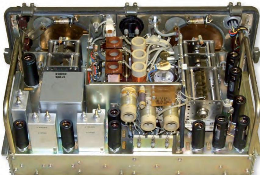
*Fig. 2: Inside the GRC-3030, the receiver is on the left and the rear panel, with the transmitter on the right and centre.*
