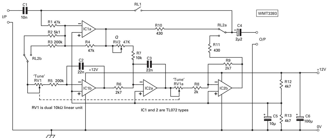
Fig. 1: The circuit diagram of the peak/notch filter, uses the quieter TL072 f.e.t. op amps rather than the original, and noisier, '741 types.
