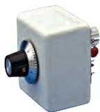
**PORTLAND VFO** as featured in March 2006 PW. 7-7.2MHz as local oscillator for a 40m direct conversion receiver or transceiver. Otherwise as 7.9-8.4MHz to use in conjunction with a mixer-vfo system as local oscillator for 4 meter receiver/transmitter with a 9MHz or 10.7MHz IF. Optional Buffer 1 for IC and Mosfet mixers, or Buffer 2 to drive a diode ring mixer. **VFO PCB with Buffer 1 or Buffer 2 PCB and parts kit with potentiometer and drilled box £23.50.**
