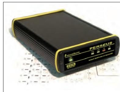
The PERSEUS r.f. analogue front-end has been designed for the most demanding users and includes a 0-30dB, 10dB steps attenuator (with an up to 500mW input lower rating), a low-loss 10 bands pass-band r.f. pre-selector filters bank and a high dynamic pre-amplifier with a top-class input third-order Intercept Point of more than 30dBm. The resulting third-order dynamic range is 103dB for s.s.b. signals (2.4kHz bandwidth) and 107dB for c.w. signals (500Hz bandwidth).
