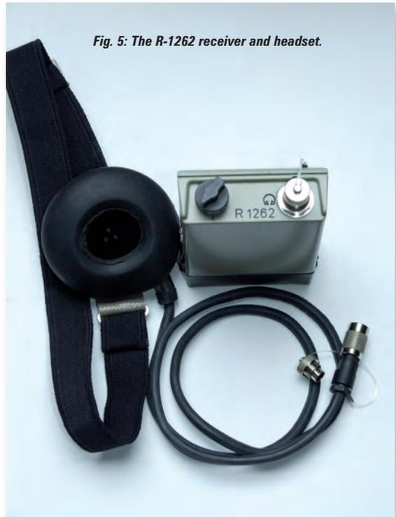
**Fig. 5:** The R-1262 receiver and headset.
