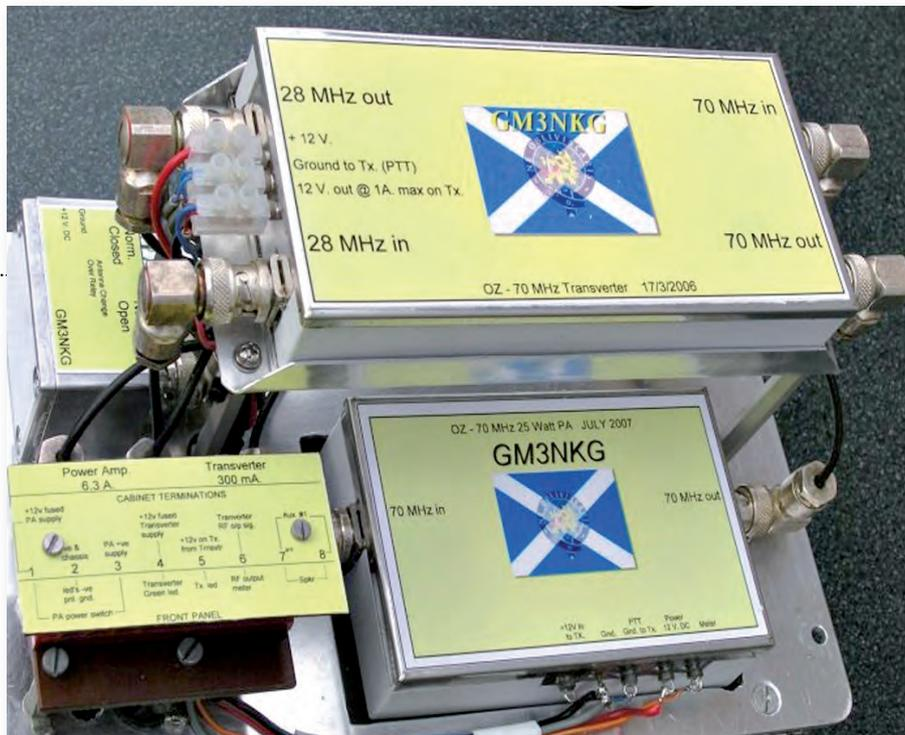
Fig. 1: The 70MHz transverter constructed by GM3NKG.
