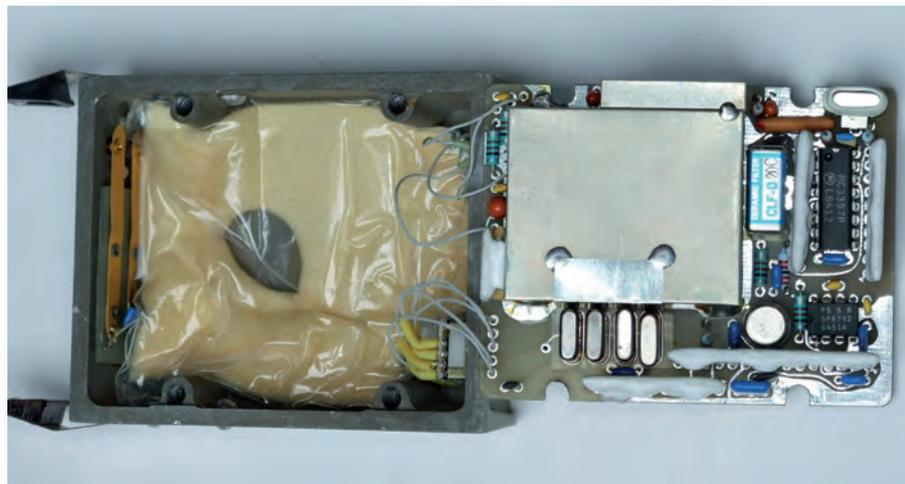
**Fig. 6:** Inside the R-1262, a compact design, with the four crystals visible on the lower left.
