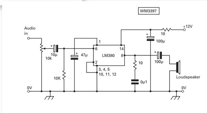
Fig 1: Typical circuit diagrams for either the LM380 or the LM386 are shown here.
