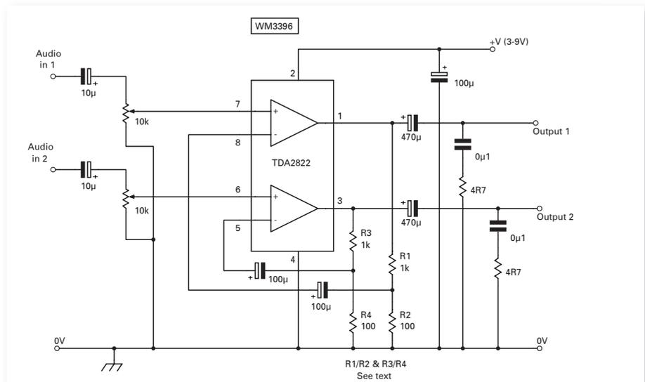
**Fig. 4:** The diagram shows a stereo amplifier with some external feedback, provided by resistors R1, 2 and R3, 4. Using the feedback resistors the gain is adjustable from about 10 to 100 times.
