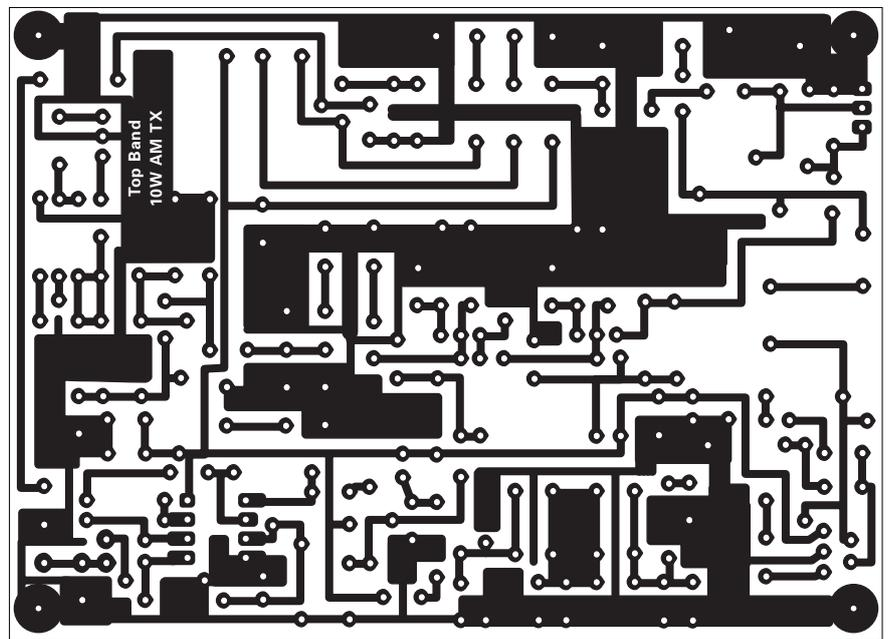
Fig. 2: The final p.c.b. layout artwork and component placing.
