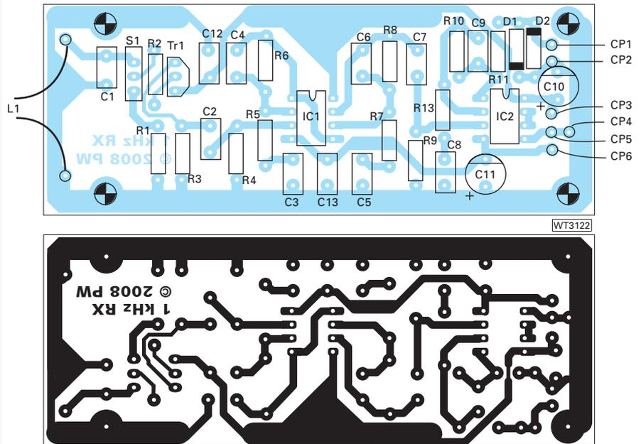
Fig. 2: The p.c.b. artwork diagram and overlay of Ted's 1kHz receiver.
