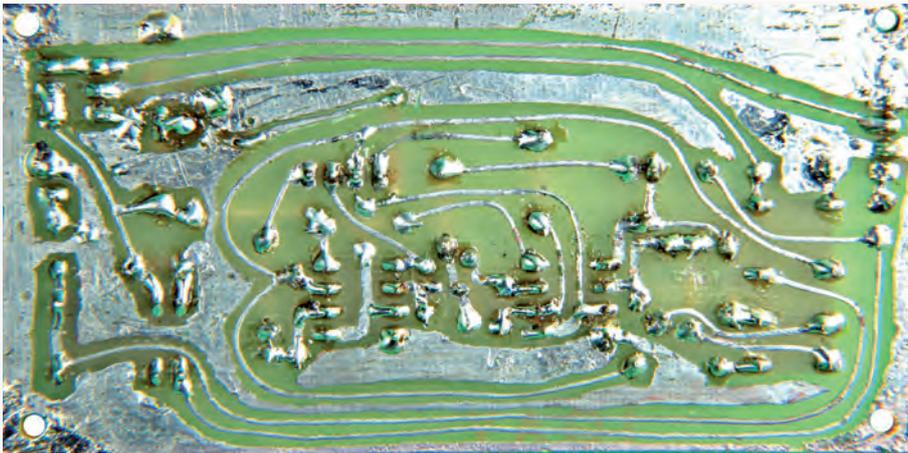
Fig. 3: The track pattern of the prototype.
