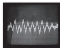
Waveform of received 1kHz, mains harmonics.
