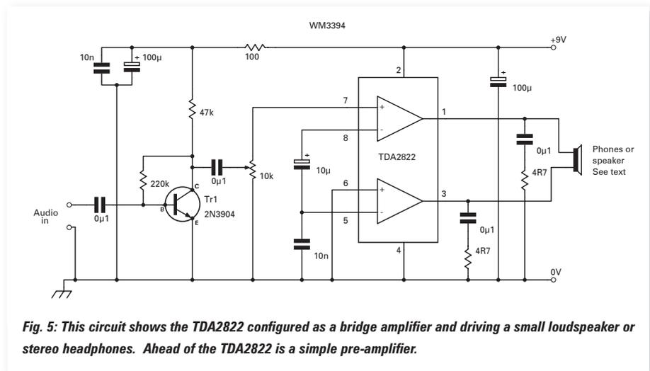
**Fig. 5:** This circuit shows the TDA2822 configured as a bridge amplifier and driving a small loudspeaker or stereo headphones. Ahead of the TDA2822 is a simple pre-amplifier.
