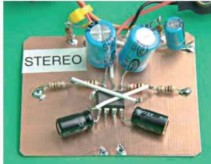
*The stereo version of the TDA2822 utilising feedback as in Fig. 4.*
