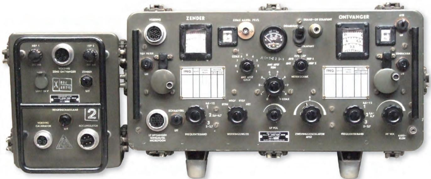
*Fig. 1: The GRC-3030 with dynamotor (motor-generator) power supply.*
