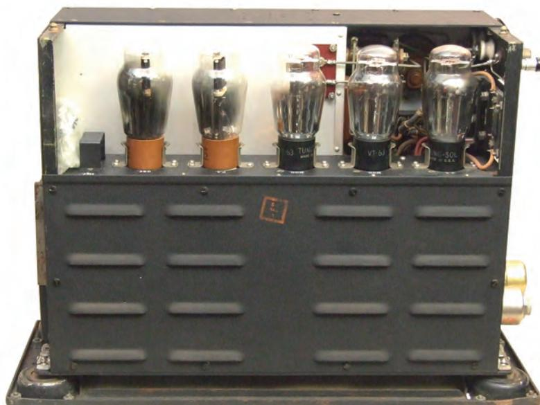
Fig. 4: The valves inside the BC-223-AX transmitter, easy access if replacement needed.
