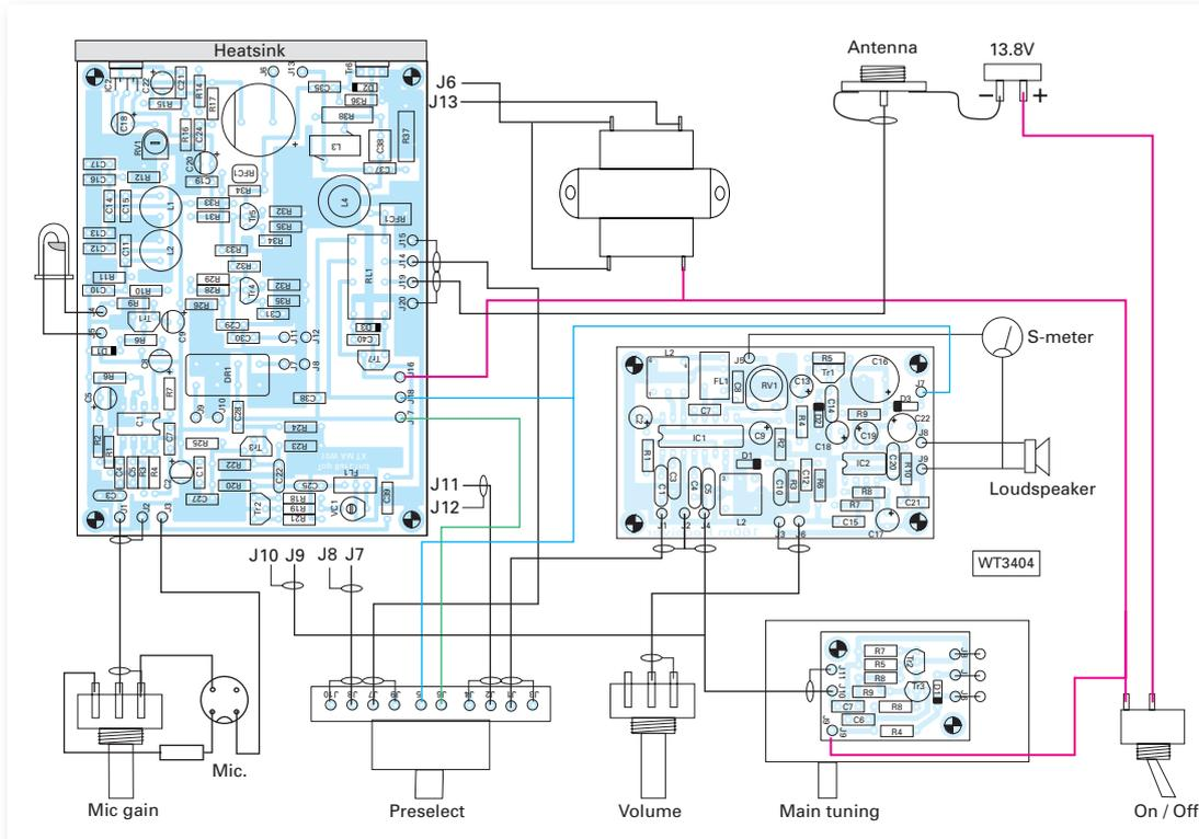
Fig. 3: Diagram showing all modules of the 1.8MHz project that make a complete transceiver.
