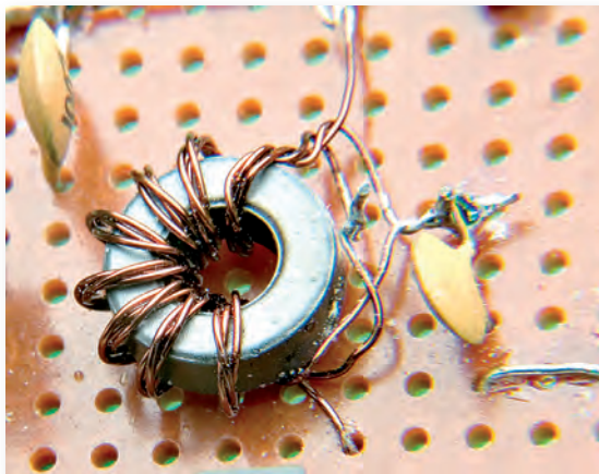
The detail of the trifilliar-wound toroidal transformer and the layout of the whole project below.
