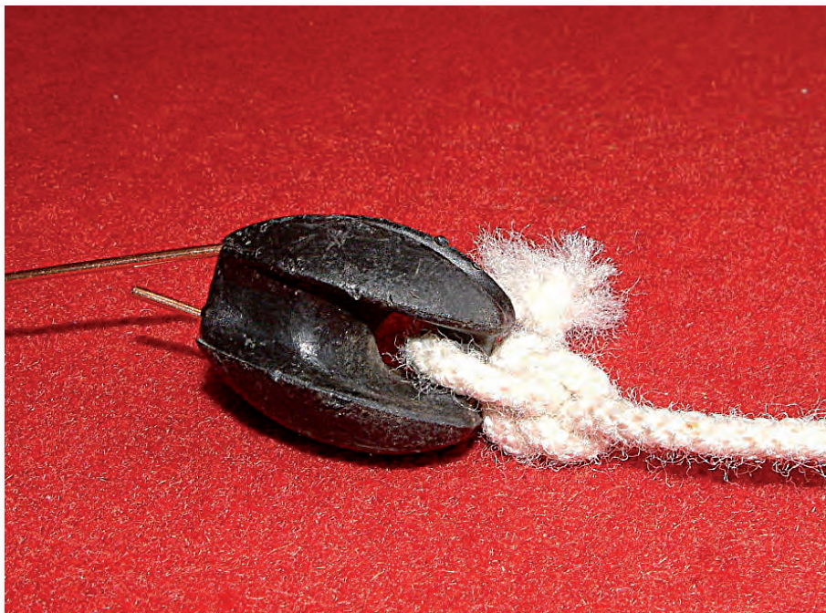
This picture should make it apparent how to use the egg-insulator at the ends of a dipole. In reality, this rope would become a little less effective as an insulator in wet weather, due to water retention. A polypropylene rope would be rather better.
