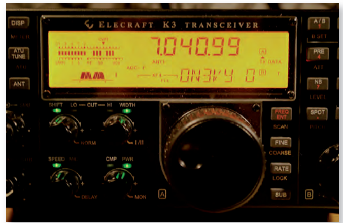
Decoded RTTY signal from ON3VY on K3 showing decoded callsign scrolling across lower part of display. Note the two peaks of the dual-tone FSK filter shown in the lower left of the screen. Above that the CWT display shows the correctly tuned-in RTTY with roughly equal numbers of bars in the \pm parts of the display.
