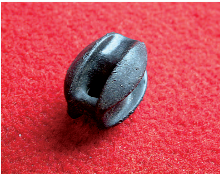
Made from plastic now, rather than from porcelain as used to be the case, this antenna end-insulator has two holes set at right-angles to one another. This type of end-insulator is often called an 'egg-insulator'.
