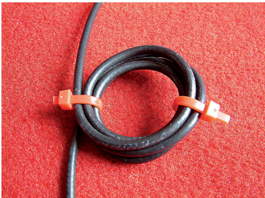
An effective choke-balun for the higher h.f. bands can be made in coaxial feeder, simply by creating a five or six turn loop of about 100-150mm in diameter. To make an effective choke-balun for the lower h.f. bands, use 10-12 turns with the same diameter range.
