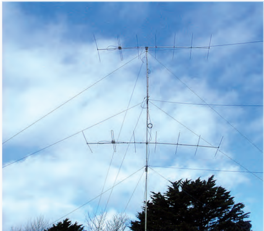
Fig. 1: 70MHz antennas at G4ADV/P 2 x 7-element Yagis Photograph by Kevin Franks M0BFB
