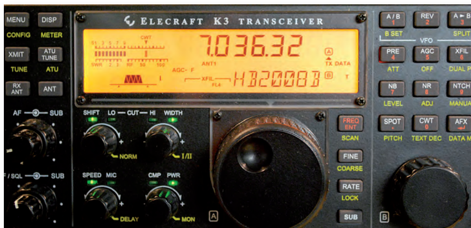
Decoded BPSK 31 signal from HB2008B on K3 showing decoded callsign scrolling across lower part of display. The CWT display shows a single bar in the centre indicating a correctly tuned-in signal.
