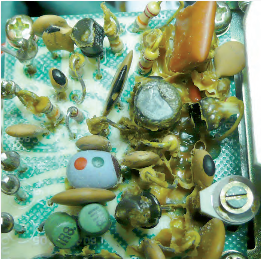
Fig. 3: After some hard work with fine-nosed pliers and a small heat source, the glue can be removed, which often seems to improve the frequency stability.
