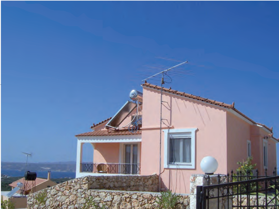
Fig. 1: The 50MHz and 70MHz antennas at the QTH of J49K in Crete was being operated by Martin Platt G4XUM.
