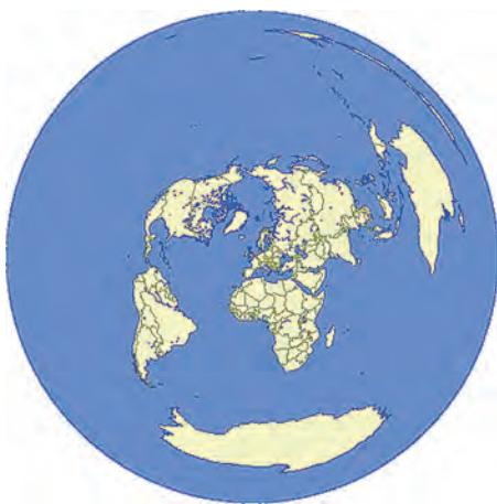
Fig. 5: A Great Circle map shows the direction of the shortest path to anywhere else in the world, but the countries look very distorted. This map is based on path direction from UK stations to be found at the centre if this map. Great circle maps for other countries will look very different!
