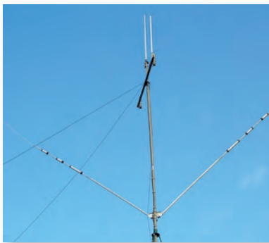
Fig. 2: The Comet H422 in use at G3LDI – shown erected in a low 'V' format.
