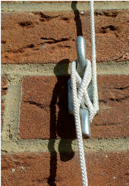
Fig. 2: A galvanised 'cleat' hook (used for washing lines) is an ideal way to tie-off the antenna halyards.
