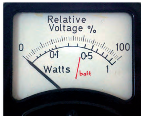
Fig. 3: An r.f. voltmeter with power scale.
