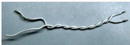
Fig. 2: A home-brewed 'gimmick' capacitor made from insulated and twisted wire.
