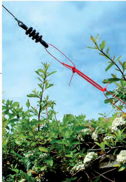
Fig. 3: Cable ties are very useful for use on antennas. They are tough and don't lose their strength quickly due to 'bleaching' due to the ultra-violet rays from the sun.
