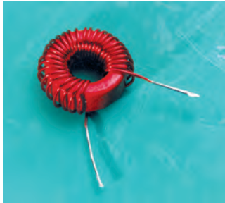
Fig. 1: Winding a toroid - spacing of the wire endings is important (see text).
