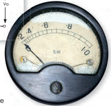
Fig. 4: An r.f. ammeter showing square law scale.
