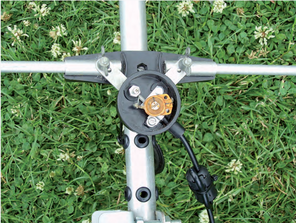
Fig. 4: Andy replaced the coaxial cable stub with a trimmer.
