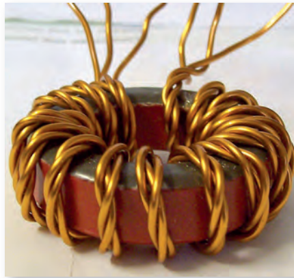
Fig. 5: The toroid form of balun wound on a suitable toroid core.
