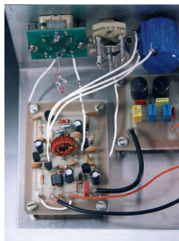
Fig. 5: Close-up of the main receiver p.c.b. of the receiver. The 'pig nose' ferrite bead transformer (described by G3RJV) can be seen mounted immediately to the left of the electrolytic capacitor in the lower centre of the p.c.b., just above the terminating coaxial connection (see text).
