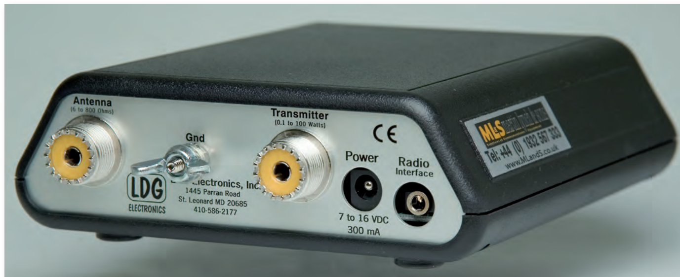
Fig. 3: As well as coaxial input and output sockets and an earthing (butterfly type) nut, there's a small coaxial power socket along with a 3.5mm jack socket (to take a stereo connected jack plug) for suitable transmitter with a 'Tune' line capability.
