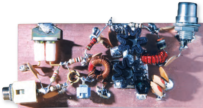
This month's project (or should it be challenge?) - features the 'mighty' 2N2222 transistor in a QRP 7MHz transmitter.
