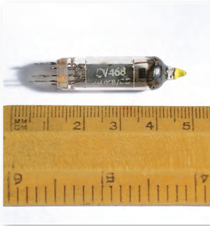
Fig. 3: The miniature wired-in EC70 valve using a 6.3V, 150mA heater and an anode dissipation of 3W.
