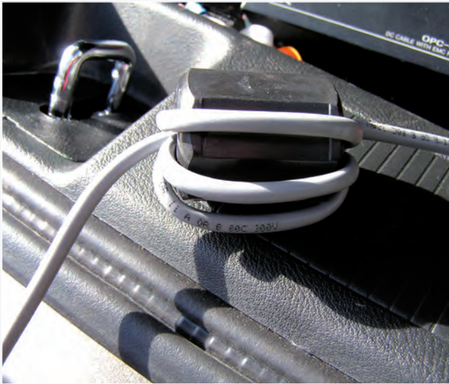
The choke must be carefully wound to ensure the motor-driver antenna works correctly.
