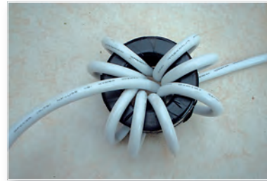
Fig. 4: Making the ferrite ring mains choke. Eight turns of mains cable (8mm dia) was wound on a pair of FT240-61 ferrite rings. This provided good choking action from 1.8 to 28MHz.
