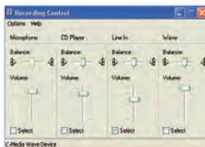
Fig. 9: The DigiPan recording control. Make sure that you tick the Select box for the appropriate slider.
