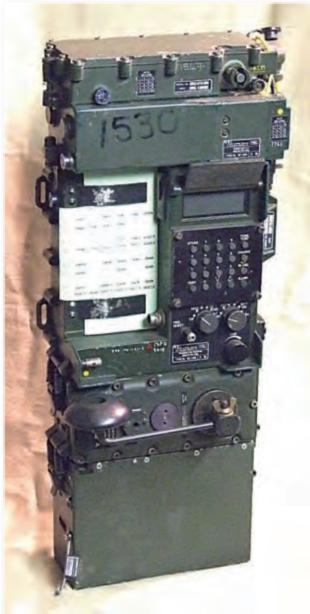
Fig. 3: The PRC-319 with hand turned battery charger fitted.
