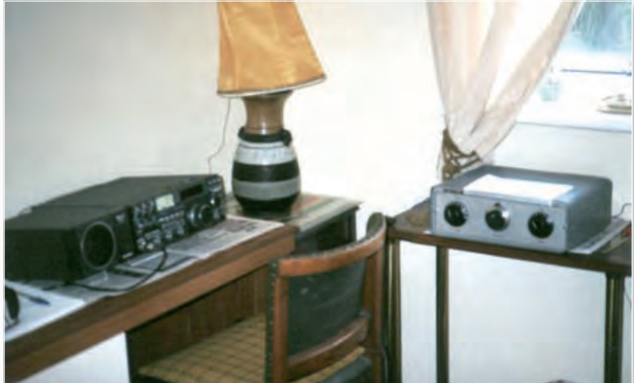
Fig. 2.1: The operating position at G3TKN/P in Cheltenham using an Icom 751A. The a.t.u. is placed near the window where the antenna enters.
