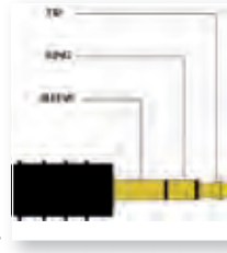
Fig. 6: A typical 3.5 Stereo Jack Plug. The Tip has the signal (centre of the screened lead) connected, and the sleeve has the screen connected (The ring should be left unconnected).
