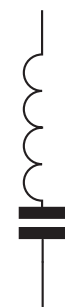
Fig. 3: Almost all capacitors look like this combination, but how do you choose the best one for the job of decoupling r.f. but not audio from microphone lines?
