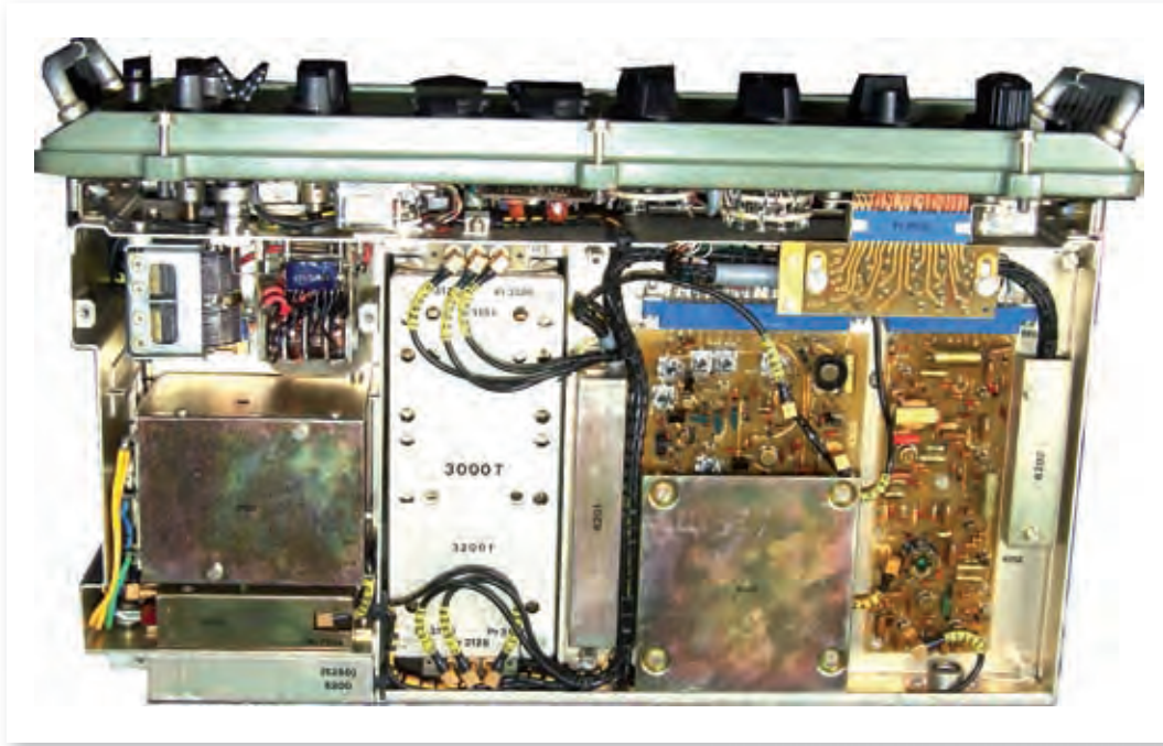
Fig. 2: Inside the RUP-15 showing the modular construction.
