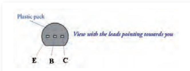
Fig. 6: The pin-outs for the BC548B transistors
