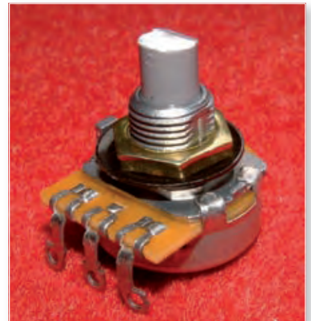
Fig. 9: The variable resistor with the spindle cut to 5mm length.
