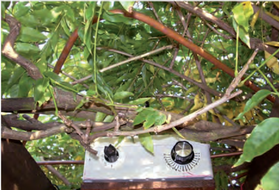
Fig. 4: The tuner and counterpoise at the top of a pergola, and hidden in a Wisteria!
