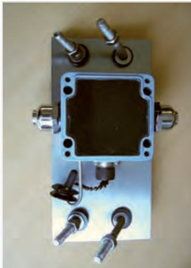
Fig. 6: The central connection box is internally filled with epoxy.
