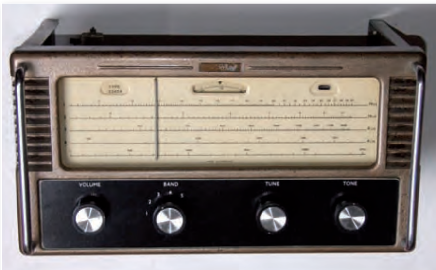
Fig. 1: The 2245A front view – the super tuning dial is typical of Eddystone receivers.
