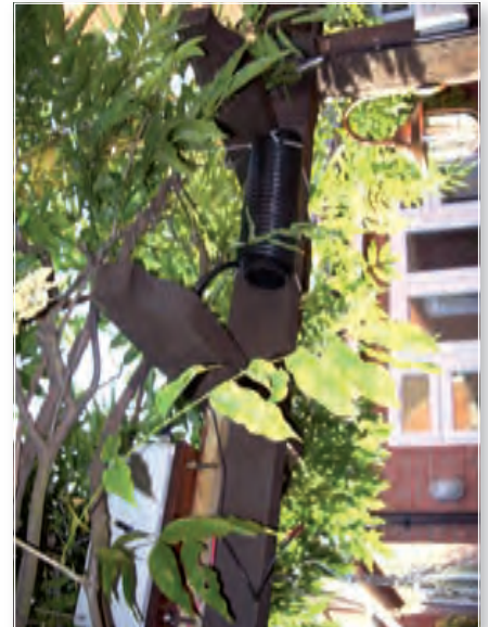
Fig. 5: The choke balun runs down, and is attached to a leg of the pergola.
