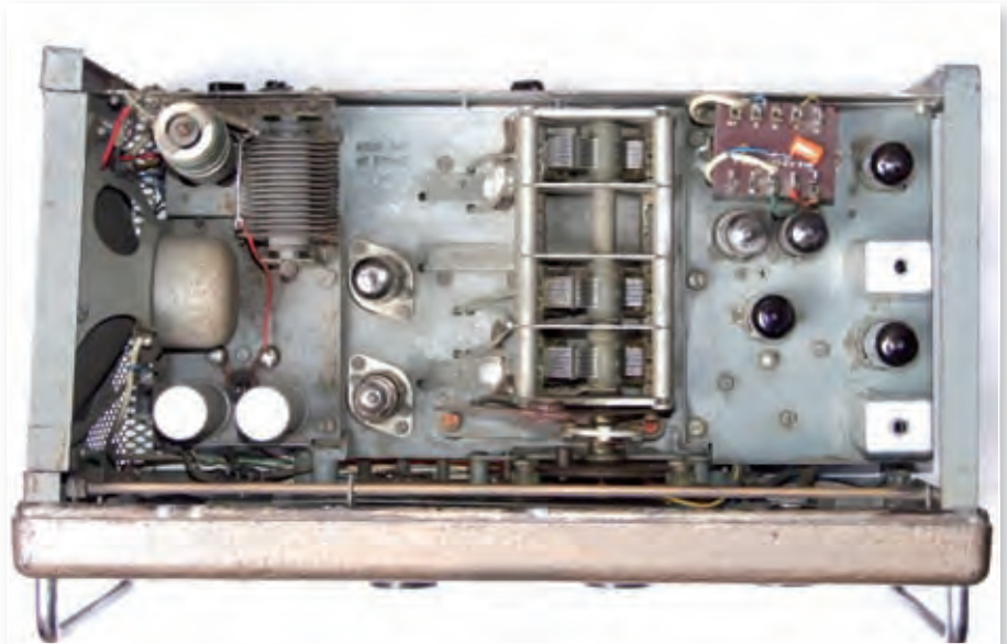
Fig. 2: Internal view of the receiver, with the p.s.u. on the left, tuner unit in the centre, and the i.f./audio on the right. (Note the replacement audio output transformer).
