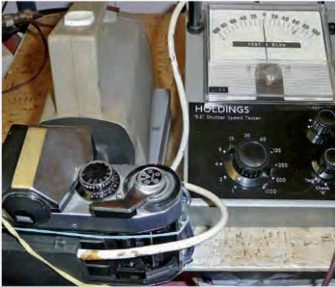
Fig. 3: The camera shutter-tester in action on the photographic test-bench.
