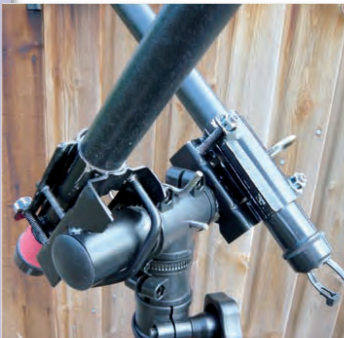
Fig. 1: The integral tripod/telescopic mast, axle head and extending arms form the support system for the wire antenna.
