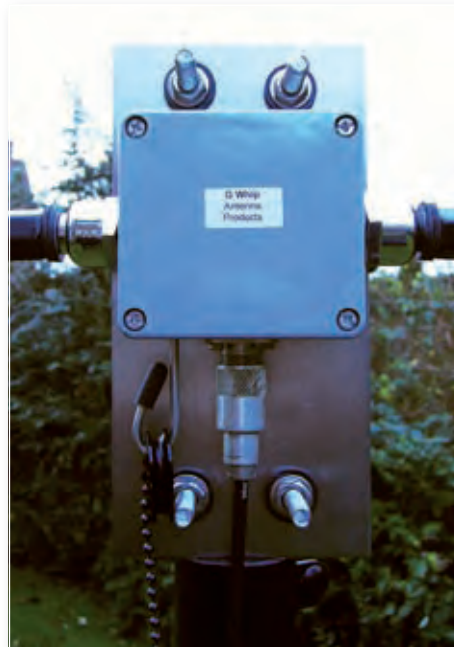
Fig. 1: The centre connection box has a coaxial cable strain relief and a coaxial cover.
