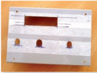
Fig. 3: An 'Abra-file' sawblade make the job of cutting 'letter-box' hole for the display, much easier.
