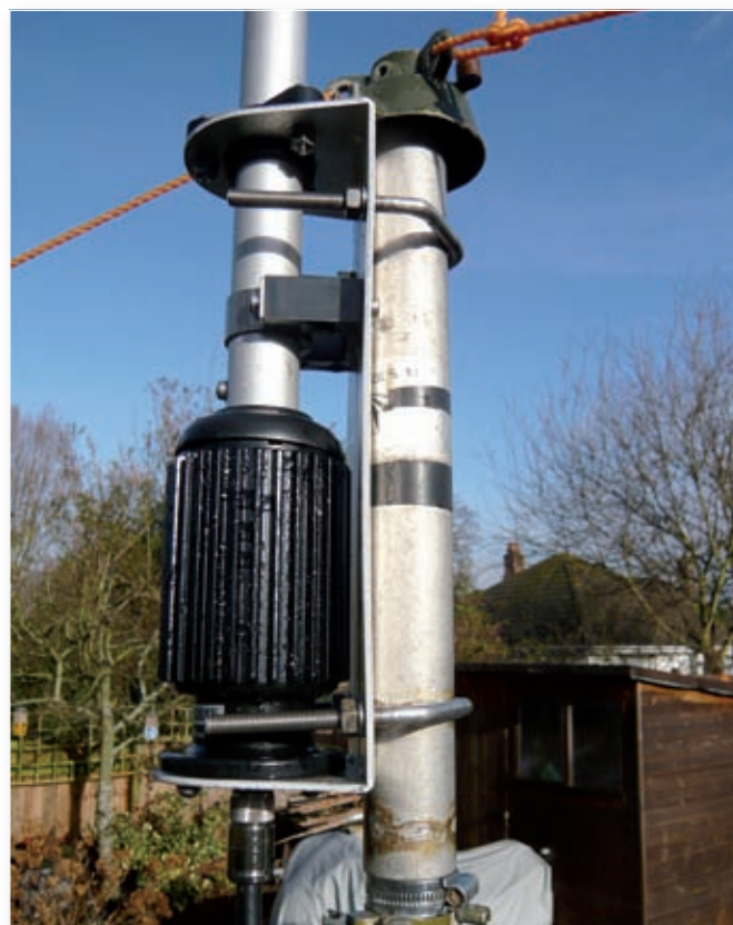
Fig. 1: This is the feed-point of the antenna, showing the matching section and the clamp fitting onto a mast.
