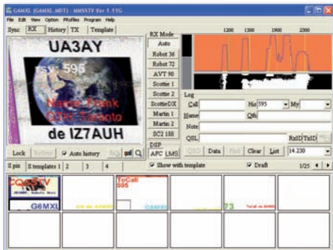
Fig. 6: Receiving First Picture – note the slanted verticals.
