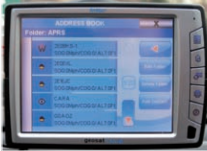
Calling up the APRS folder within the in-built address-book allows you to choose locations via the touch-screen.
