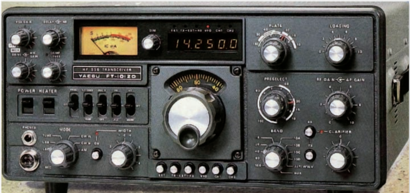
Fig. 2: The original Yaesu FT-101ZD had neither a.m. or f.m. but adding them could cause problems with earth loop feedback.
