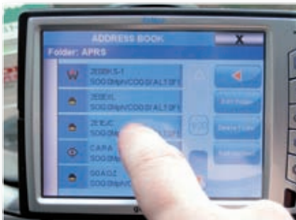
Tapping on Terry 2E1EJC's entry in the address-book selects his location as the end-point.
