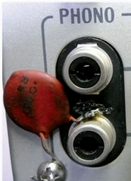
Fig. 1: An externally added r.f. filtering capacitor may be the only way of filtering some equipment.
