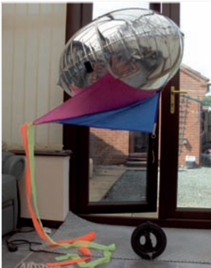
Fig. 3: A lightweight Allsopp Helikite and the reel containing the flying line/antenna element.
