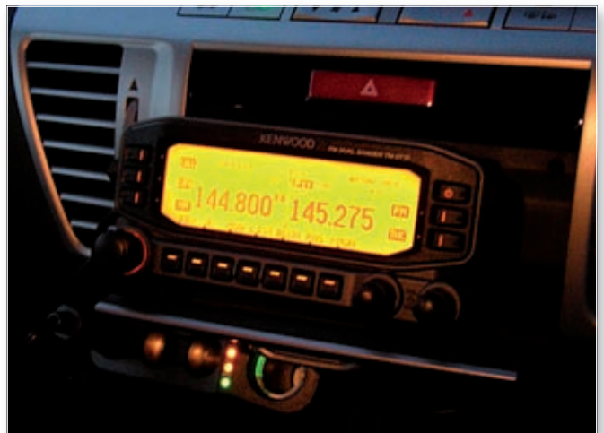
The control head for the TMD-710E was mounted on one of the small 'spare' shelves to be found on the dashboard.
