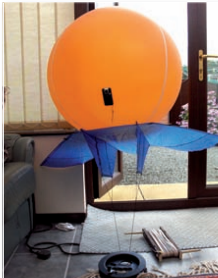
Fig. 4: The black 'mark' on the balloon is a small flycam-2 camera for taking a series of aerial photographs and storing them on a memory card.
