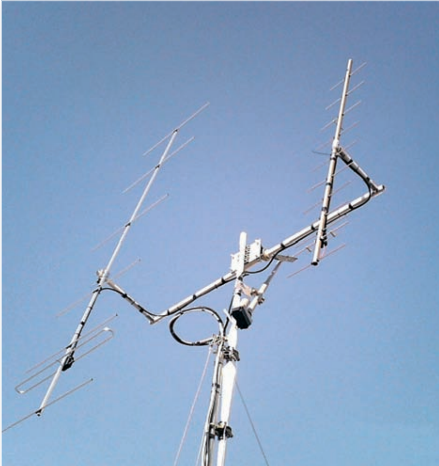
The 144MHz / 430MHz satellite antennas at the QTH of Greek station SW1JGW
