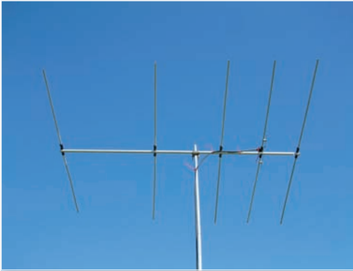
Fig. 7: A Tonna 50MHz antenna 'pruned' for 70MHz operation, by reducing all dimensions to 5/7ths of the original size.
