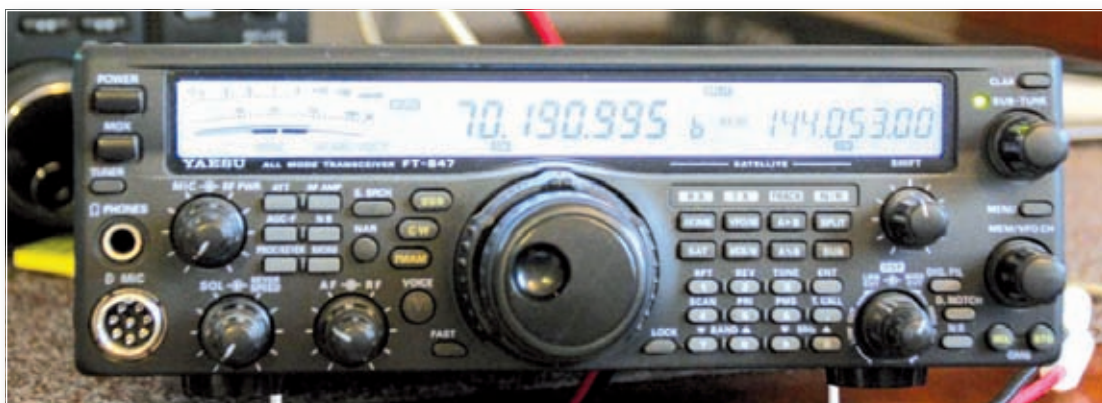
Fig. 1: The Yaesu FT-847, some versions of this now discontinued transceiver can operate on 70MHz.
