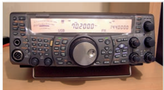
Fig. 6: The Kenwood TS2000 can configured to display the correct 70MHz frequency when used with a transverter
