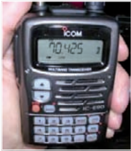
Fig. 2: The Icom IC-E90, this popular hand-held transceiver can be purchased equipped for 70MHz.
