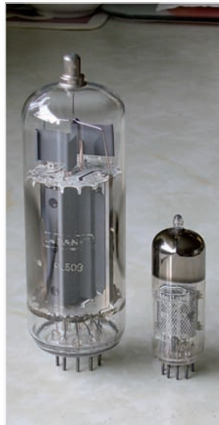
Fig. 1: PL509 and EF80 TV valves. The PL509 could be used for audio output.
