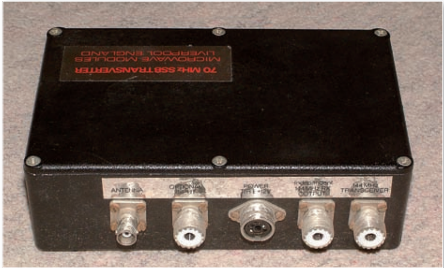
Fig. 5: The 144 to 70MHz Microwave Modules transverter, can still occasionally be picked up second-hand. There's also a 28 to 70MHz version.
