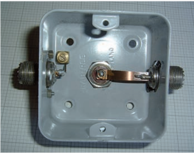
Fig. 4: The middle S0239 socket came from an antenna change-over switch, where the metal strip formed part of the switch.
