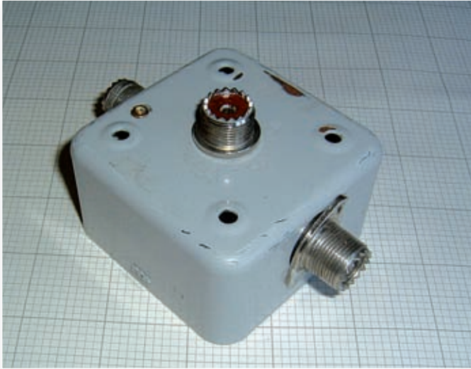
Fig. 3: After fitting the other two S0239 sockets to the patress box.
