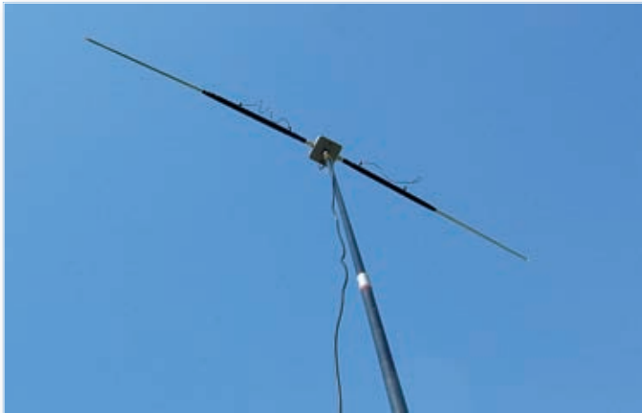
Fig. 6: Hoisted up on top one of Roy's favourite portable supports – a 'roach pole' fishing rod.
