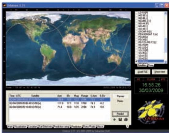
Fig. 6: Orbitron shows each pass as three lines, AOS, Maximum Elevation and LOS.
