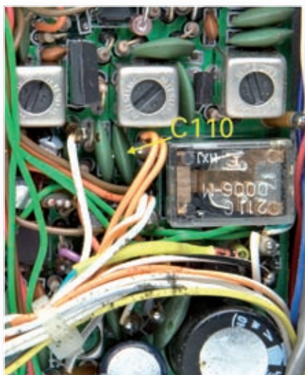
Fig 4a: Removing C110 'brightens' up the audio of an FT-290.
