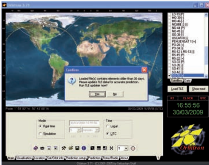
Fig. 3: A screen shot of Orbitron from the website at www.stoff.pl/ Notice how it has prompted for updates to the Keps.
