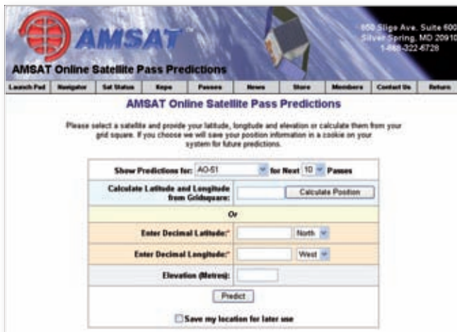
Fig. 1: A screen shot of AMSAT's online Satellite Pass Predictor. Select a satellite, enter your locator or latitude and longitude, then press 'Predict'.
