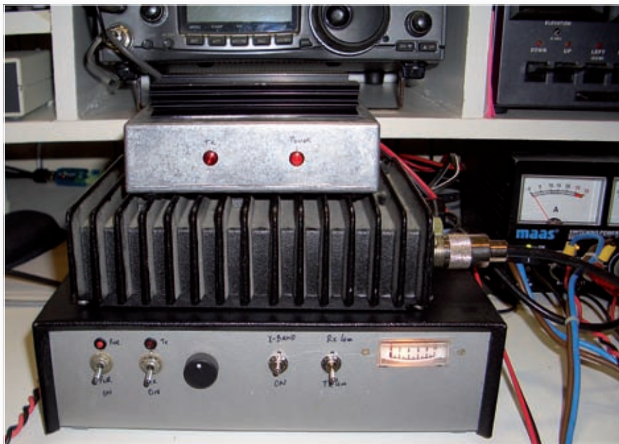
The 70MHz transverter and Pye A200 amplifier used on the Isle of Harris DXpedition.
