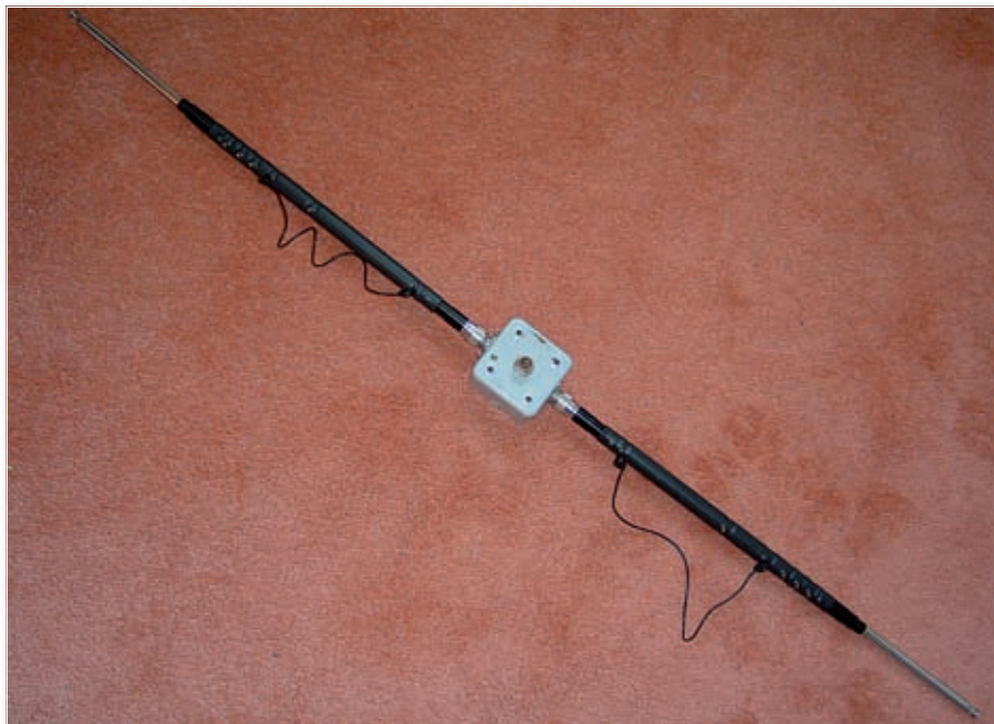
Fig. 5: The patress box with box antenna screwed into the two side-mounted S0239 Sockets.
