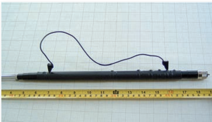
Fig. 1: There are several versions of this base-loaded multi-band antenna, that all seem to be to the same design.
