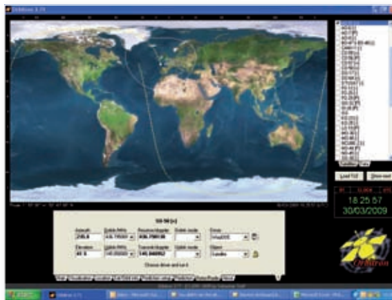
Fig. 7: Orbitron showing some of the information visible during a pass including displaying the frequency taking into account Doppler frequency shift.
