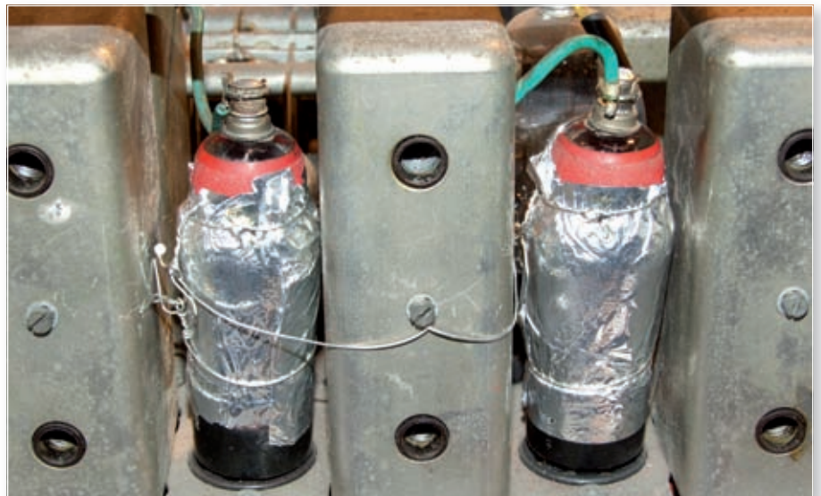
Fig. 2: The foil wrapped i.f. valves, now quietly doing their jobs!
