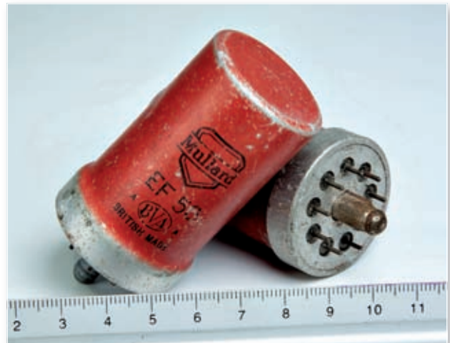
The (then) state of the art EF50 valve featured an all-glass B9G-based valve, within an aluminium screening can.
