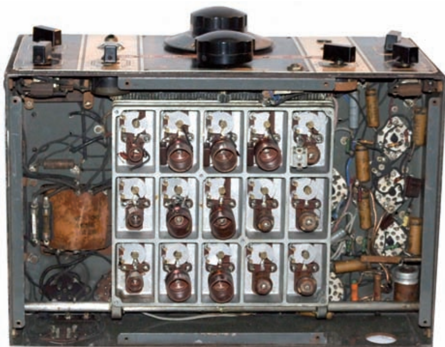
Fig. 4: The NC-100's unusual coil switching arrangement.
