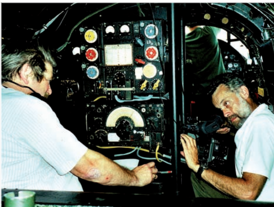
Fig. 1: Roger Hunt G3PVU in the Lancaster Just Jane being filmed for a documentary by an uncomfortable cameraman. He is sitting in front of the T1154 and R1155 wartime transmitter and receiver.
