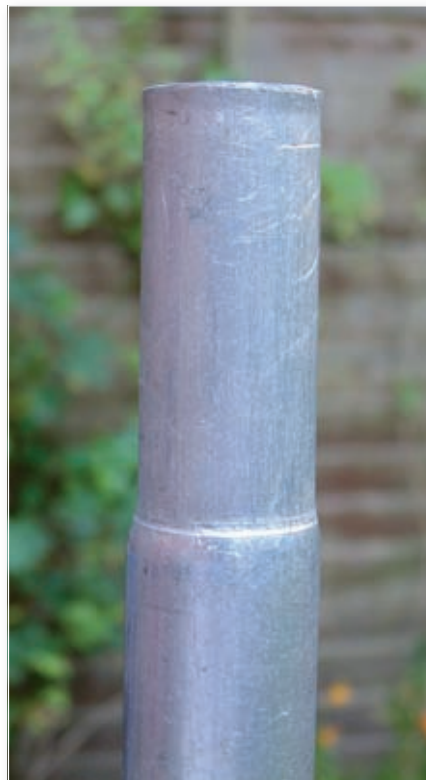
Fig. 2: An aluminium pole that has the end 'swaged' or reduced to allow it to fit inside a similar diameter pole.
