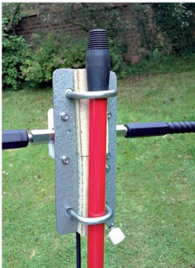
A closer look at the packing needed to allow Chris' preferred support pole to work.
