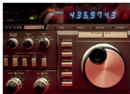
Fig. 10: The Satellite switch on Yaesu's discontinued FT-736. Note the Normal and Reverse positions for non-inverting and inverting transponders respectively.
