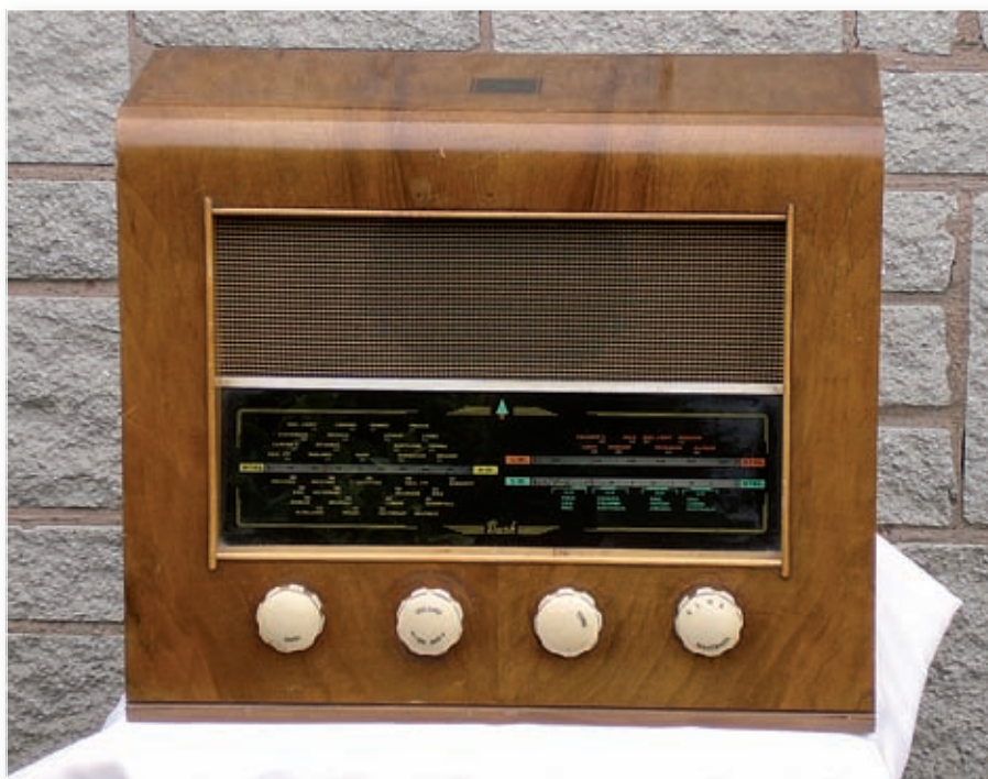
Fig. 1: A typical a.c./d.c. 'short' superhet radio of the early 1950s (it's a Bush DAC41).
