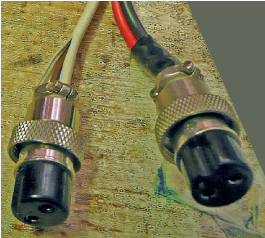
Fig. 2: These may look like they're the same, but the polarity is important too. Get it wrong by using the wrong lead and the rig could be irreparably damaged.
