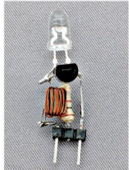
A miniature version without a p.c.b. The two pin on the plug at just 5mm apart so, you have an idea of the size of the unit.
