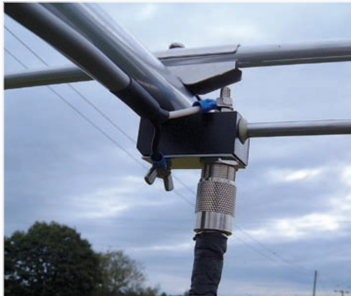
A close-up shot of the feed-point and one of the two matching elements.
