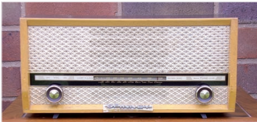
Fig. 4: A slightly larger table-top radio can show around 75% power saving by modifying the valves' heater circuitry to work on lower voltages.
