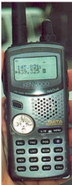
Fig. 6: The Kenwood TH-D7E dual-band f.m. transceiver can receive on one band whilst transmitting on the other band – making it ideal for f.m. satellites.
