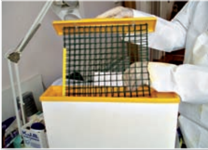
The trial p.c.b. lost within the mesh frame that holds the p.c.b. within the bubble-etching tank.
