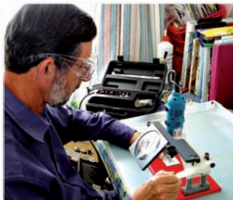
Safety glasses back on to start drilling the p.c.b. using the supplied drilling setup.
