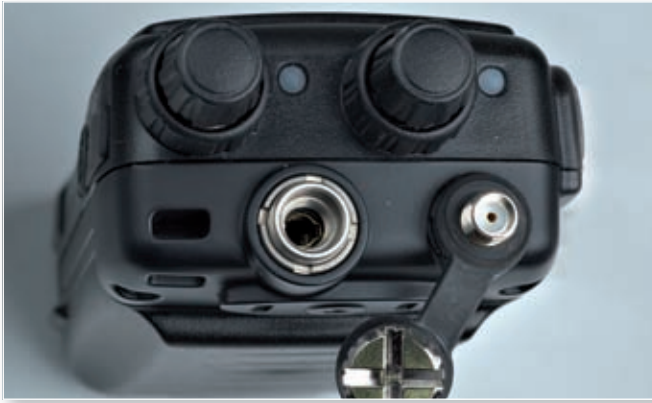
The top panel of the rig with the twin concentric controls, the SMA socket for the triple-band antenna connection and the headphone/microphone socket with its waterproof gasket and retaining screw removed.
