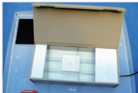
With twin ultra-violet tubes the exposure box can cope with p.c.b.s bigger than those found in most projects.
