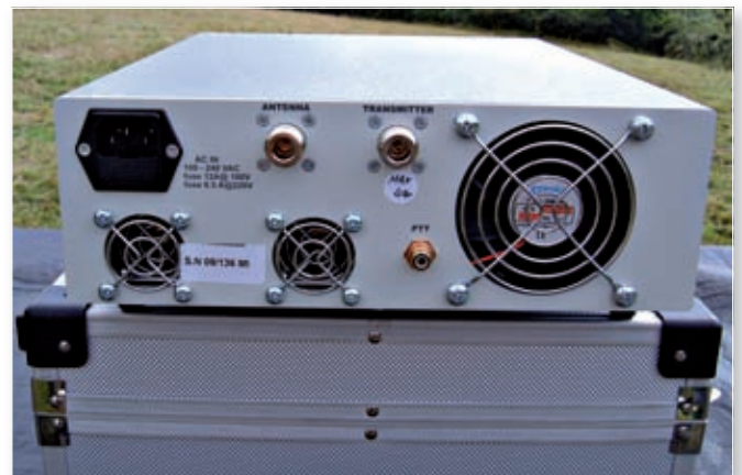
As you can see from this shot, the PSU has its own dual fans to ventilate hot air when running. The larger fan to the right is for the p.a. stage ventilation. Signals in and out of the amplifier, go via good quality N-type sockets.
