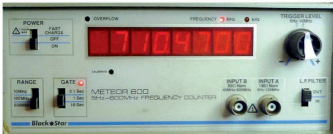
Fig. 3: Although very effective as a pure frequency counter, the Black Star Meteor 600 counter cannot directly display the frequency that a transceiver's dial is set to.
