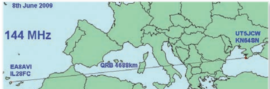
Fig. 2: One contact on June 8th, the 4688km path of the contact between EA8AVI and UT5CJW.
