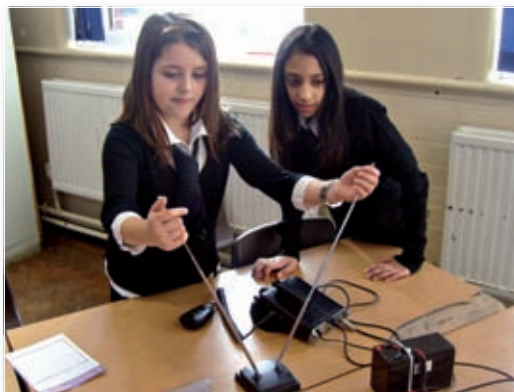
Leia and Henna adjusting an antenna for minimum v.s.w.r.
