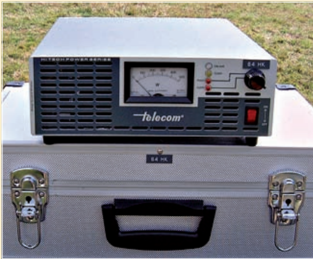
Sitting on top of its padded interior smart aluminium carry case, that's used to transport the Telecom 64-HK 50–70MHz dual-band linear amplifier.
