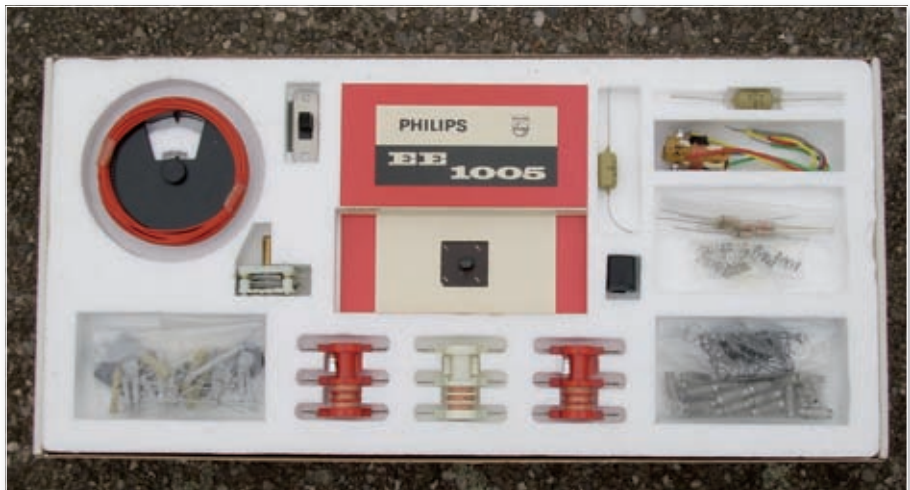
Fig. 4: The Philips' electronic construction kit add-on kit contained enough components to make a superhet radio.
