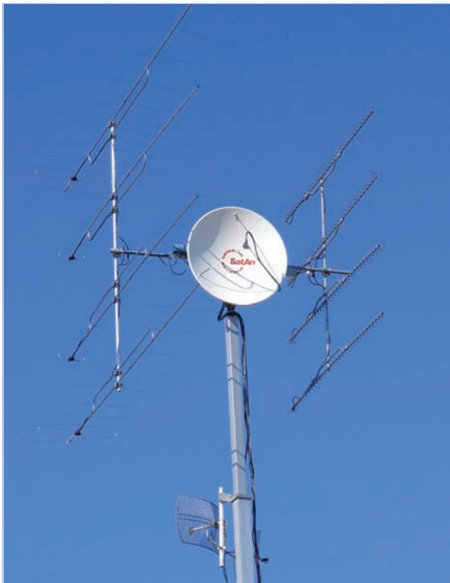
Fig. 2: The v.h.f., u.h.f. and microwave antennas at the QTH of Wolf-Henning Rech DF9IC.
