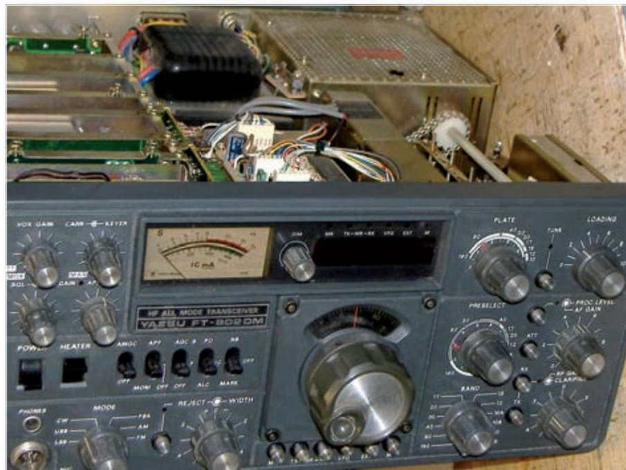
Valved h.f. rigs such as this FT-902 can have problems if it hasn't been switched on for years!
