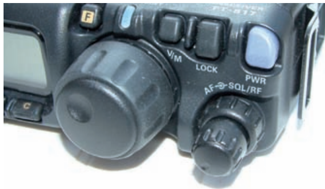
Fig. 6: Part of the front panel of the FT-817 with the blue On-Off button marked PWR and the volume (inner) and squelch (outer) dual concentric controls below.
