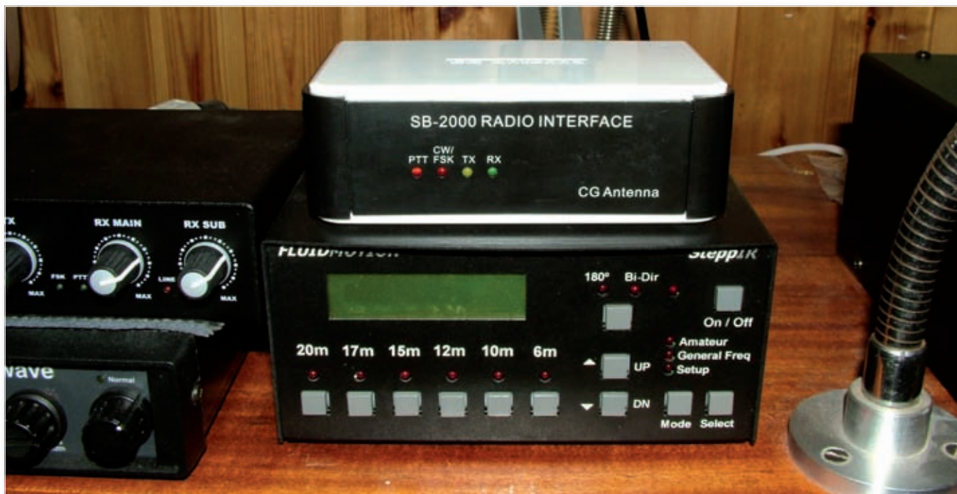
Fig. 2: In its normal operating position, other than the four activity l.e.d.s, there's little to look at on the SB-2000.
