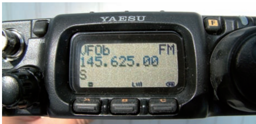
Fig. 7: The main display of the FT-817 with the Power Output display at the bottom.
