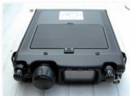
Fig. 2: The battery compartment on the bottom of the FT-817.
