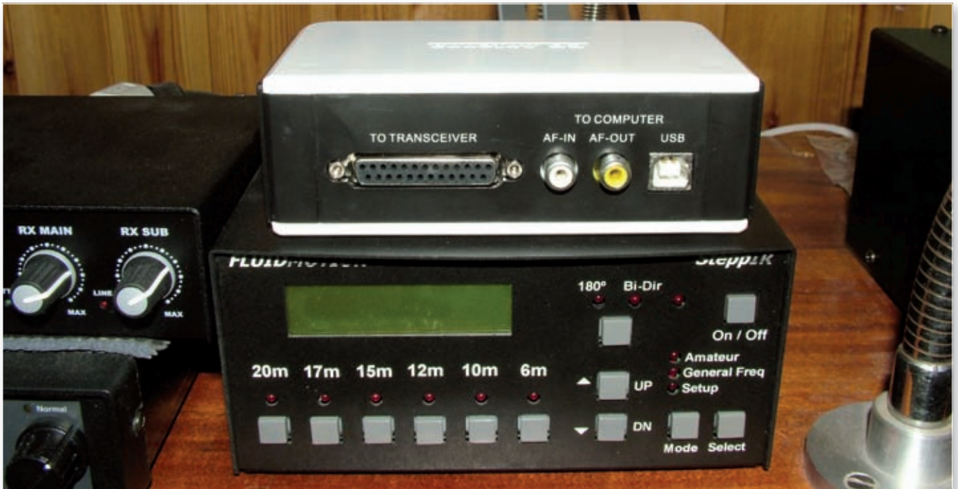
Fig. 3: Just four connectors on the back panel, three to and from the computer and the large 'D' type connector to the radio, via a rig-specific set of cables.
