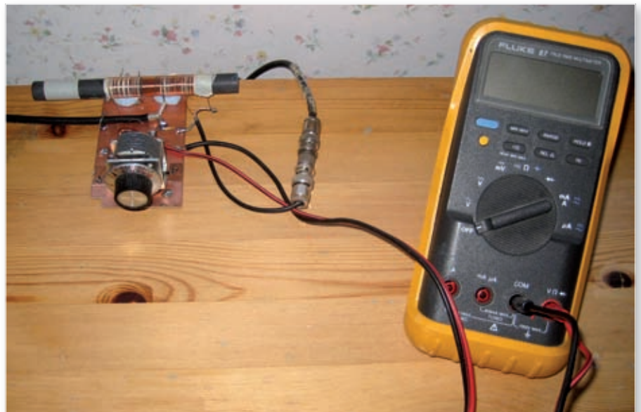
Fig. 3: Initial tests were carried out with this antenna tuning unit, constructed from a ferrite rod from a medium wave radio, wound with around 100 turns of 0.2mm wire.
