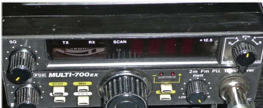
Fig. 1: Tony’s FDK-700EX 144MHz rig worked satisfactorily from 144 –145MHz, but was ‘dead’ in the top half of the band. Find out what Harry did to resurrect it!
