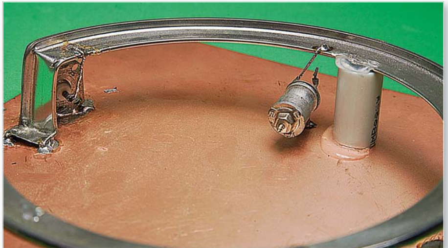
Fig. 7: The 'beehive' trimmer is around 30pF at maximum, but only a few picofarads were required to tune the antenna, when mounted around a quarter of the way around the loop as shown here. Moving the position closer to the feed-point would mean more capacitance was needed to achieve resonance.
