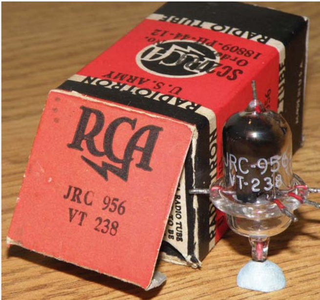
Fig. 4: Photograph of a 956 acorn valve, with its JRC-956 and VT-238 numbers helpfully printed on the valve itself and on its box.
