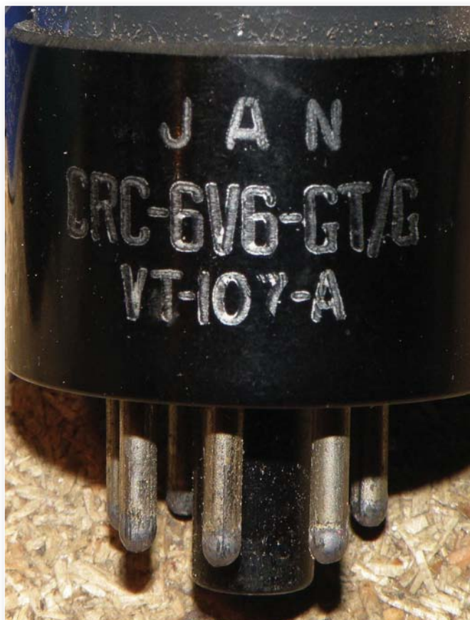
Fig. 3: Photograph of the JAN-6V6 valve showing how this code appears on the base of this valve.
