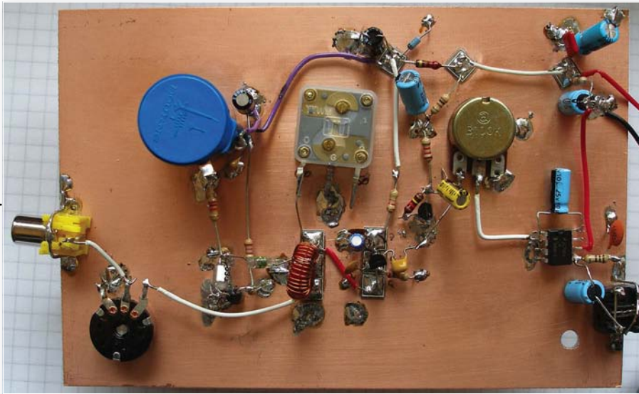
All the components are mounted 'dead-bug' style on the rear of the front panel made from copper-coated board, forming an 'earth-plane'. The layout follows the circuit diagram, with the antenna input on the left-hand side, audio output on the right.
