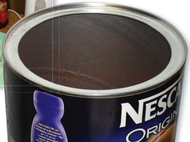
Fig. 1: When on coffee-duty at the Poole Radio Club, Tex started thinking about the possibilities of using the top of the coffee tin as an antenna. With a diameter of a little under 160mm, the outer circumference is around a quarter-wave on 144MHz. Time to let the mind wander round a few possible design shapes. Well it has to be round – doesn't it?
