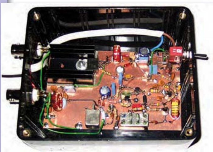
Fig. 1: The new transverter in its box provide a full 5W output from a single IRF510 f.e.t.
