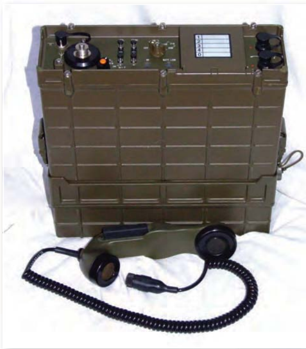
Fig. 1: The SE6861 transceiver and handset with 30V battery pack attached.
