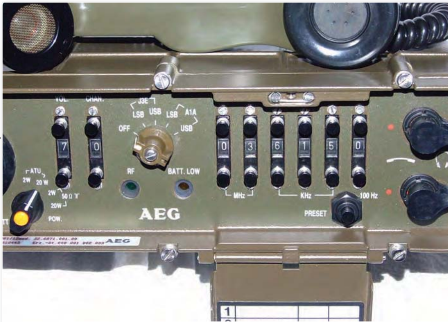
Fig. 3: Close view of the tuning and function controls.
