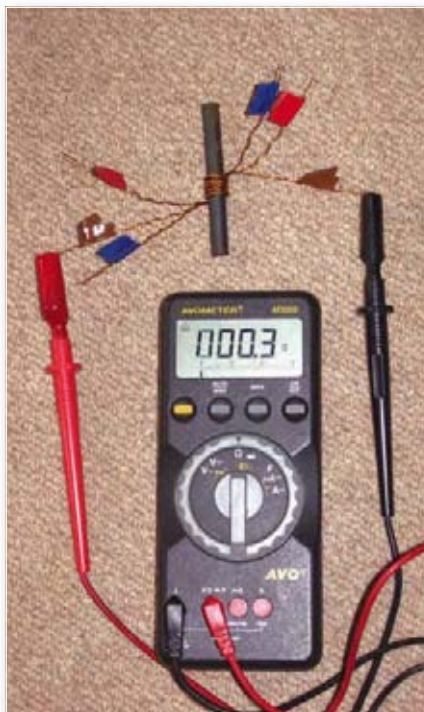
Fig. 2: After winding six turns of the composite 'wire' on the ferrite rod, the individual ends are identified and labelled.
