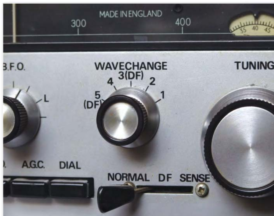
Fig. 6: The Direction Finding control.
