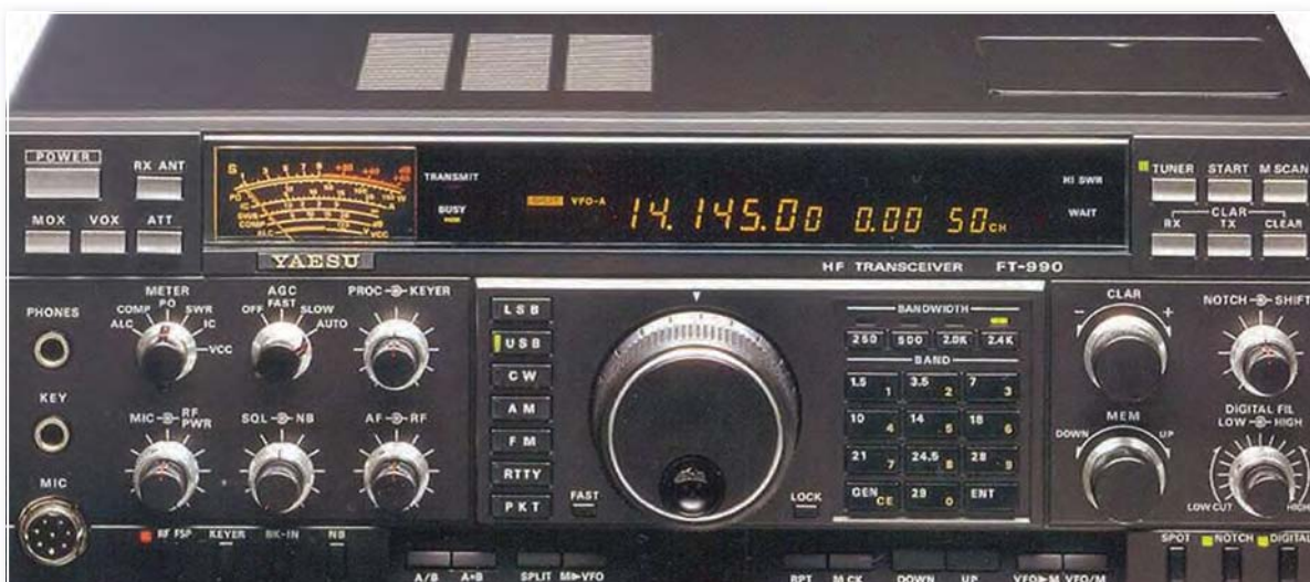
Fig. 1: The Sell-and-Forget FT-990, had a peculiar place for the RX ANT switch, just to the right of the main power switch (top left of the front panel). If you turned the rig over, it was easy to inadvertently press this on, switching antennas on receive.
