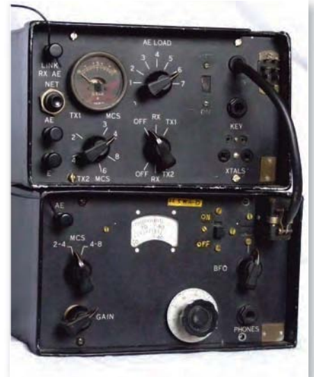
Fig. 4: The Mk128 transmitter (top) and receiver.
