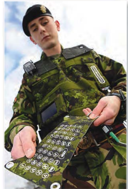
Fig. 1: A fabric which can store and conduct electricity is being developed, your clothing could even be used as an electronic keyboard (Photo credit: Ministry of Defence)
