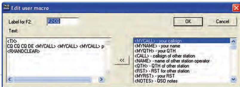
Fig. 2: Selecting the MYCALL option from the right-hand pane to build a Macro by highlighting it and 'clicking' the << button.
