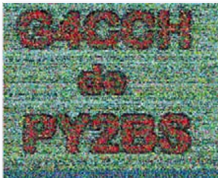
Fig. 2: Slow Scan Television signal received by G4CCH via moon-bounce on the 1.3GHz band.
