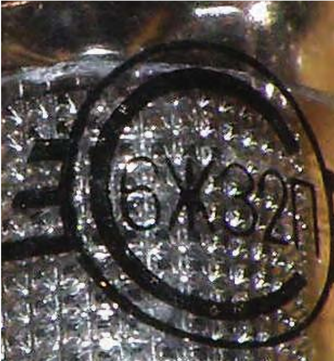
Fig. 5: My 6Ж32I1 valve showing how the Cyrillic code appears on the envelope of the valve.
