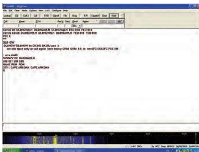
Fig. 1: Digipan following installation. It is possible to allocate macros to each of the buttons near the top from Lookup to Multi and label them as you wish.
