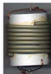
Fig. 9: A trap is just a parallel tuned circuit, however it's created.
