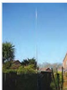
Fig. 10: The Comet H422 rotary trapped dipole (used in a V form in this photograph) antenna for 7, 14, 21 and 28MHz. It can be used either 'flat' ordinary dipole form) or in the V form as shown.
