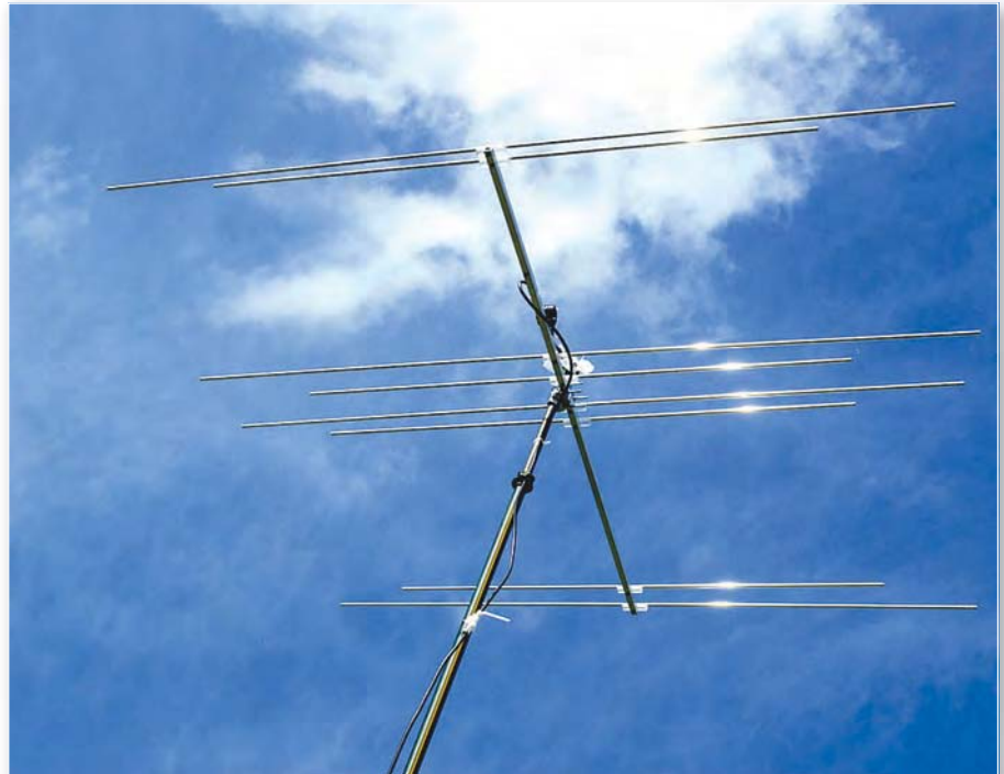
Fig. 1: The dual-band Yagi antenna designed by Justin Johnson G0KSC for use on both the 50 and 70MHz bands.
