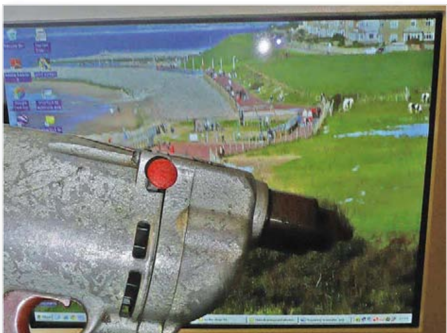
Fig. 1: Using a drill can be a useful tool to fix colour 'splodges' that sometimes appear on older, but otherwise still useful monitors. But it is a 'non-contact' fixing method! My screen (shown) survived the drill treatment!
