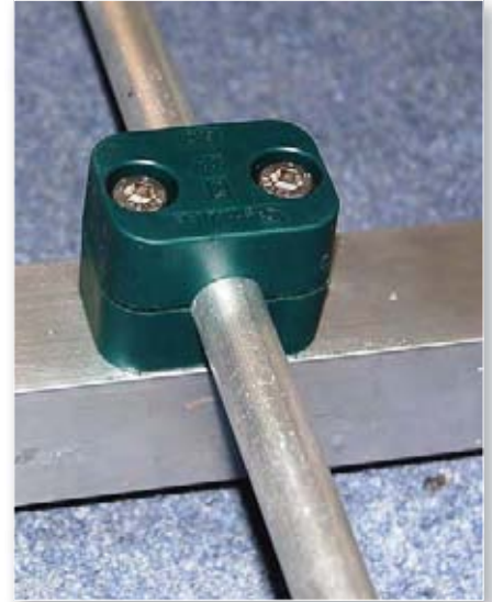
Fig. 3: All elements in this design are insulated from the main boom using specialist insulators, that can be obtained from Justin GOKSC.
