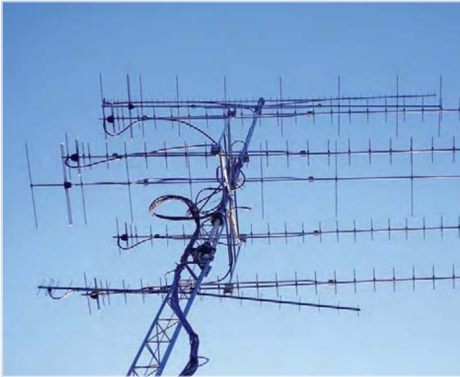
Fig. 2: The 430MHz antennas at the QTH of Reg Woolley G8VHI.
