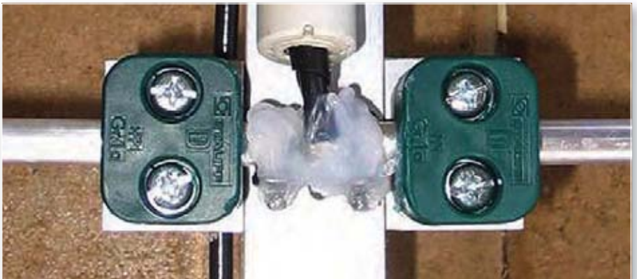
Fig. 5: 50MHz driven element is best supported by two insulators as shown here before and after weather sealing.
