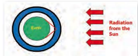
Fig. 2: Sunspots cause higher levels of ionisation in the ionosphere (shown in blue) which refracts h.f. radio signals back to earth.
