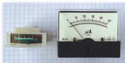
Fig. 6: two meters that George has found suitable for his s.w.r. and power indications.
