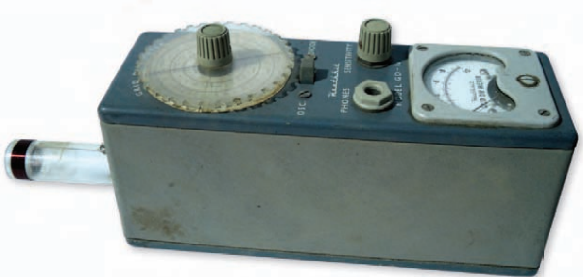
Fig. 1: A grid dip oscillator, would have originally had a valve as the active device in the oscillator, but new versions will have an f.e.t. or transistor instead.
