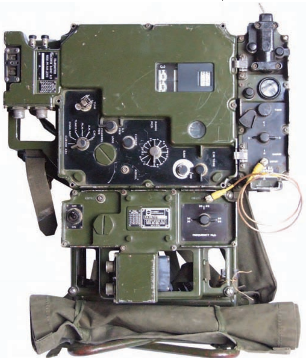
Fig. 1: The A13 on its carry frame, set at the top, amplifier below with antenna tuning unit on the left.
