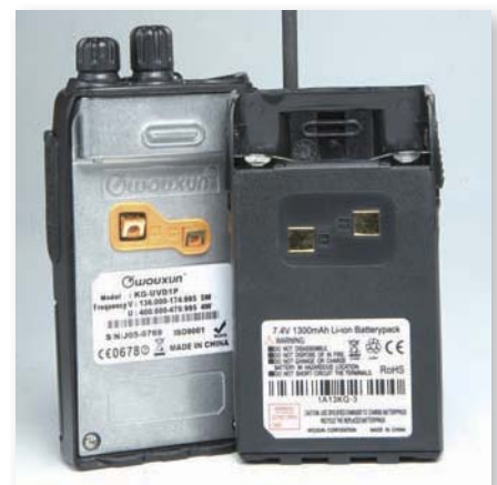
Fig. 3: The battery pack clips securely to the metal-framed unit, and is released by the action of two slide-buttons at the same time.
