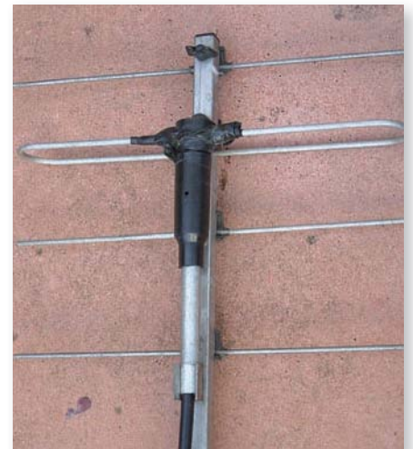
Fig. 4: A sleeve or bazooka balun as implemented by Tonna on one of their 432MHz antennas. Note the use of self-amalgamating tape to waterproof the connections.
