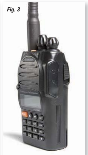
Fig. 3: The extension speaker/microphone sockets are behind a close-fitting seal on the right-hand side of the rig. The button behind is one of two that allow the battery to be released.
