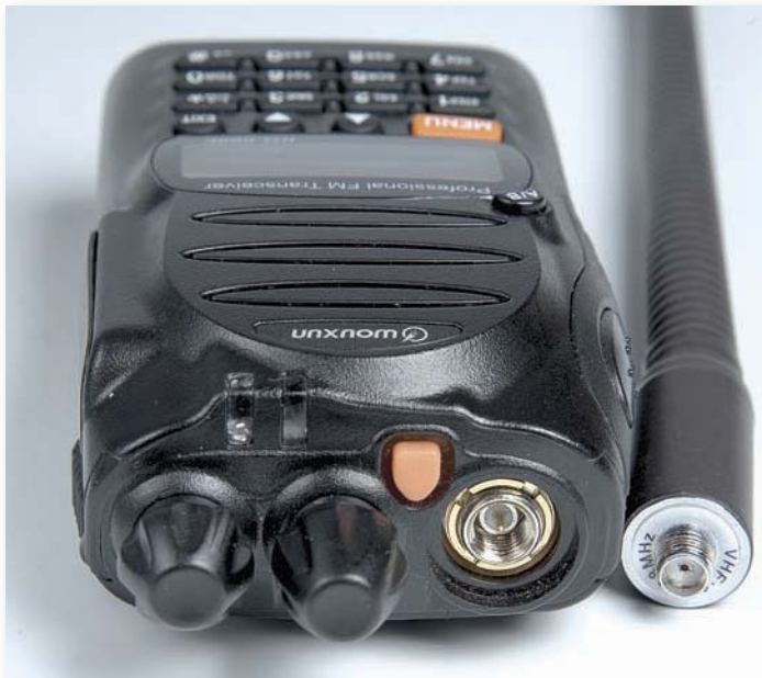
Fig. 4: The unusual combination of free SMA socket on the bottom of the antenna and matching fixed SMA plug on the body of the rig.
