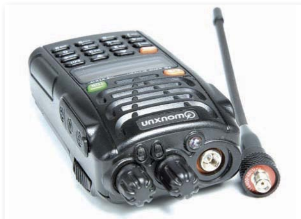
Fig. 2: The unusual SMA plug and socket arrangement for the antenna. The I.e.d. on the top panel doubles up as a torch, when its control button is pressed.
