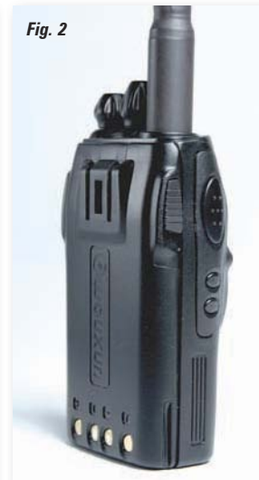
Fig. 2: The push-to-talk switch is accessible to the index finger of a right-hand user.
