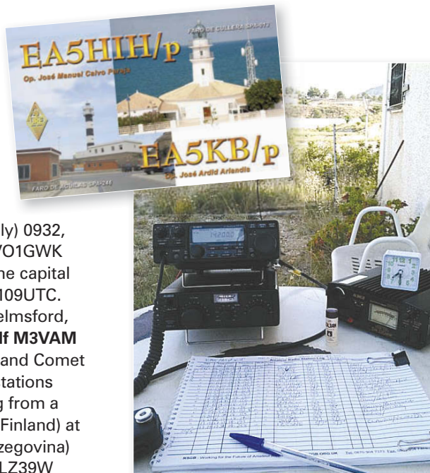
Martin Juhe operated in Spain from La Romana near Alicante as EA5/M0XJP and running an Alinco DX-70TH at 75W and EDX-1 tuner to a full size G5RV.
