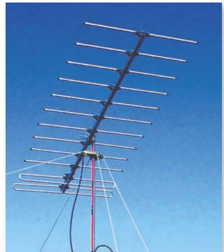
Fig. 8: A ZL-Special antenna, made popular by the late Fred Judd G2BCX in his many articles in PW .
