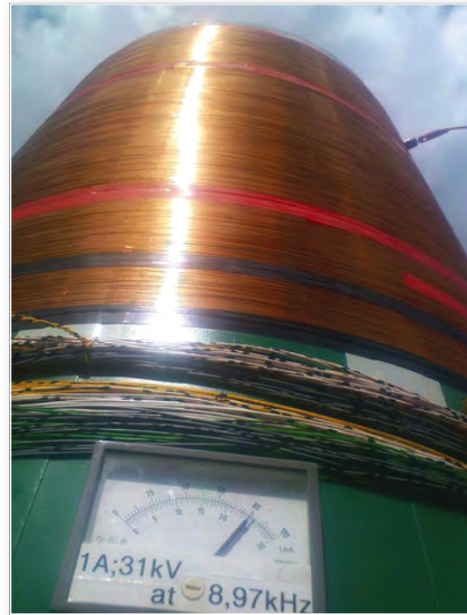
The huge loading coil used by Stefan DK7FC for 8.97kHz. Shown in his electrically quiet mobile location and close up.
