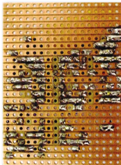
Fig. 3: Mike's sketch and photograph of the underside view of the layout of his version, built on Veroboard.
