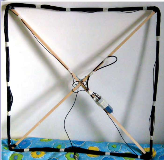
The G3XBM v.l.f. receiver 800mm square, 30-turn, loop antenna, shown here with a v.l.f. - h.f. up-converter.
