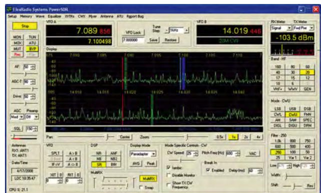
The 'radio' is controlled and driven from the control and monitor screen. So, the radio can be upgraded, merely by changing the software.
