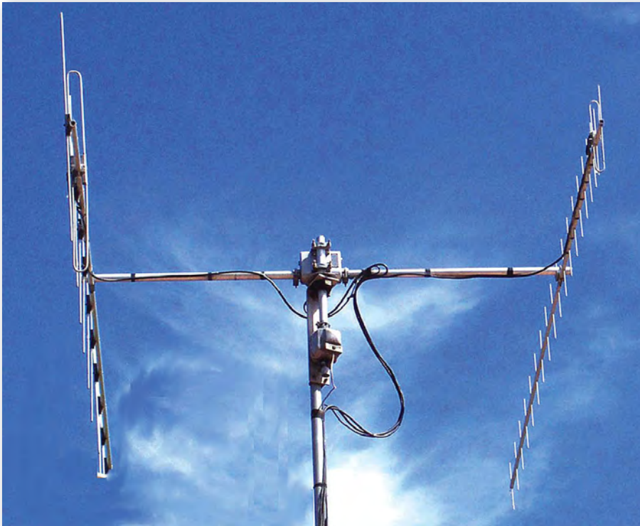
Fig. 5: A basic satellite set-up with separate azimuth and elevation rotators.
