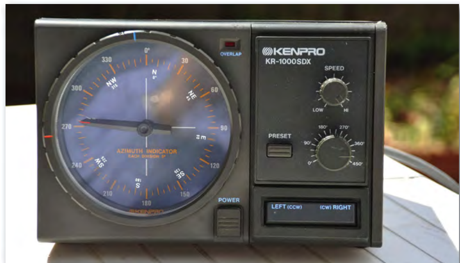
Fig. 4: Control box for a Kenpro KR-1000SDX 450° azimuth rotator. Here the overlap has been set between west and north. Note: The Kenpro range is now sold under the Yaesu brand.
