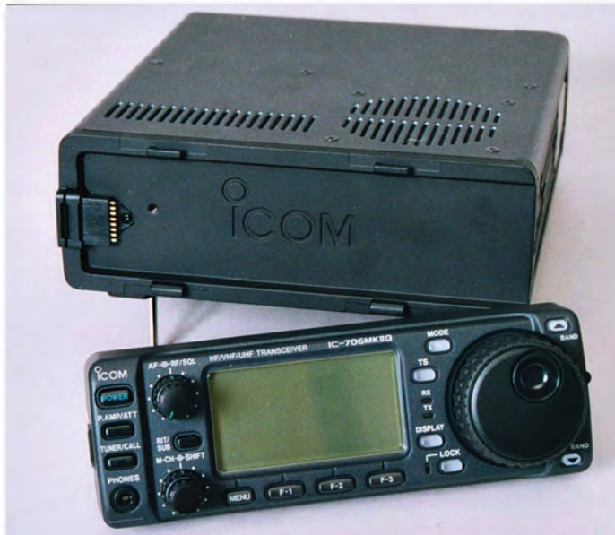
Fig. 4: As with the Alinco DX-70, the IC-706 series can have a remote location for the control head, making it easier to remove the unit, when not in use.
