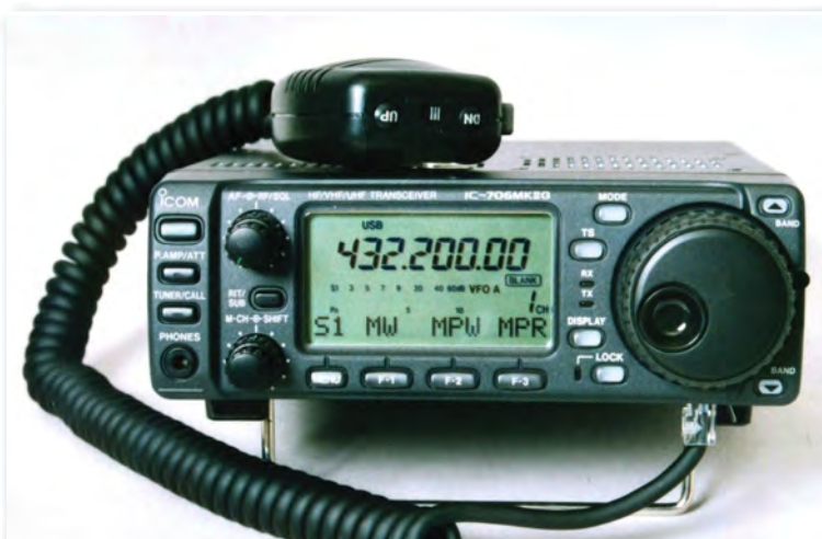
Fig. 5: The IC-706MkIIIG offered operation on the major Amateur bands from h.f. to u.h.f.
