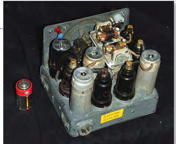
Fig. 4: Inside the RSI-4T, with six valves squeezed in easily.
