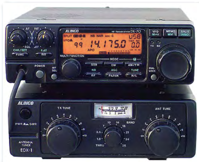
Fig. 1: The original Alinco DX-70 with its matching antenna 'tuning' unit.
