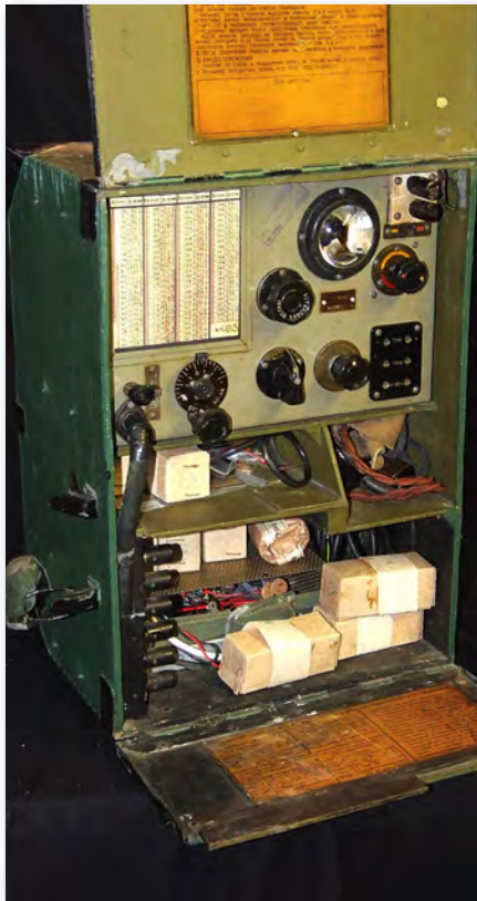
Fig. 1: The 13P backpack set in its wooden case.
