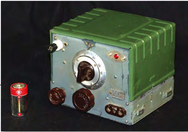
Fig. 3: The RSI-4T miniature receiver, with C cell by the side.
