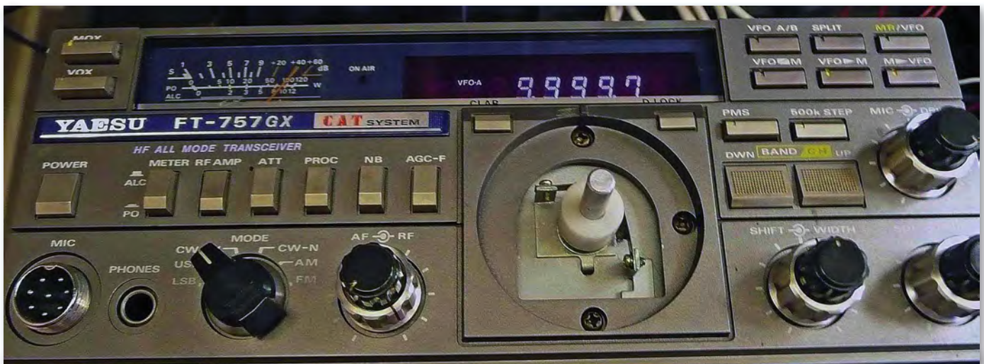
Fig. 3: Removing the knob of the FT-757 and the plastic sleeve, on the tuning control allows you to apply a little WD40 liquid to ease a sticky main shaft bearing.
